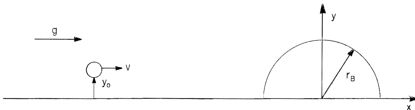
Figure 1.—Geometry of a single-bubble, single-particle system, where g is the force acting on the system, v is the velocity of the particle, y_0 is the initial position of the particle, and r_B is the radius of the bubble.
