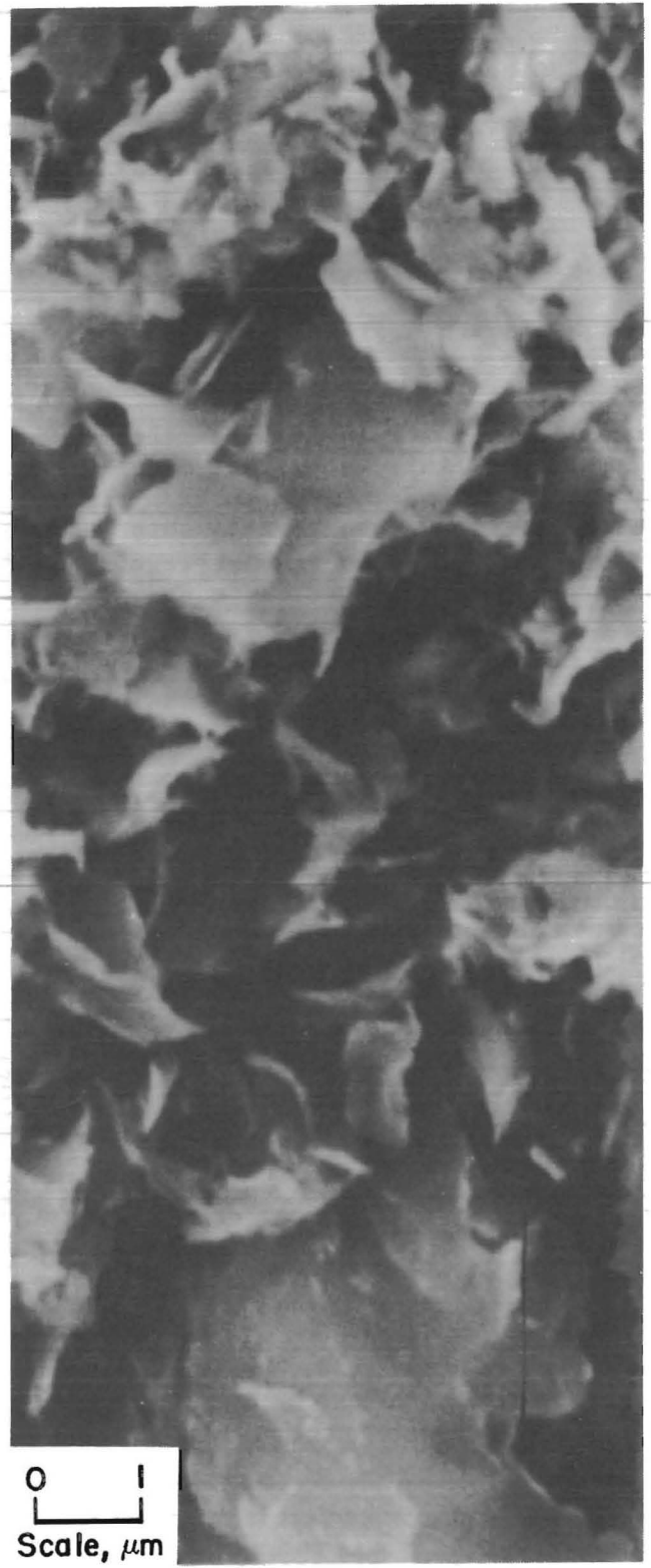
FIGURE 10. - Photomicrograph of Ba-exchanged montmorillonite dewatered by PEO.
