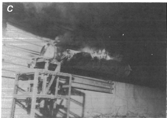
FIGURE 8.—In-mine fire test of duct D. A, Setup; B, 2.5 min after ignition; C, 3.5 min after ignition; D, duct after test showing extent of flame damage.
