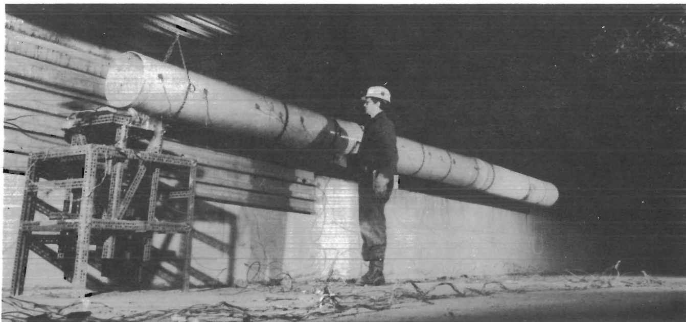
FIGURE 7.—Test arrangement for full-scale in-mine fire tests of ventilation ducts.
