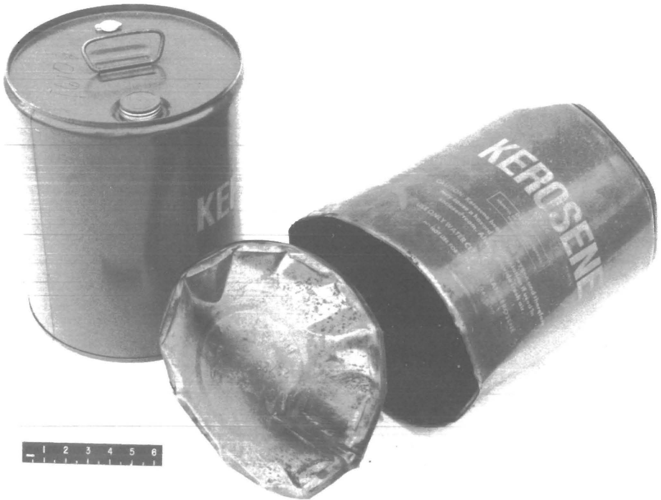
FIGURE A-10. - Vented dark blue containers before and after standard tray fire (kerosene contents) showing bottom blown off by explosion of kerosene vapor and air.
