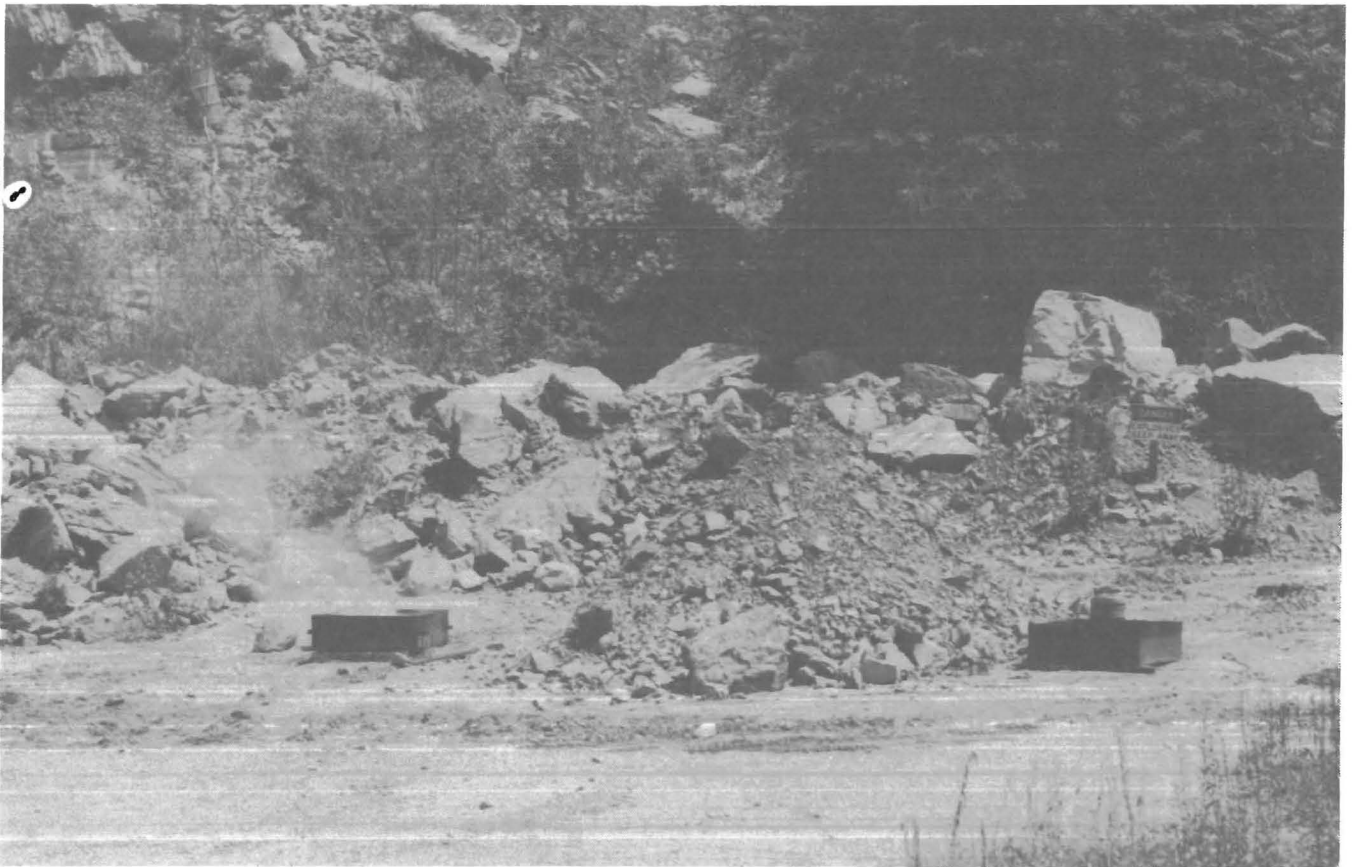
FIGURE 4. - Tray fire test showing intact metal safety container (right) after 7 min and fire-consumed plastic container (left).
