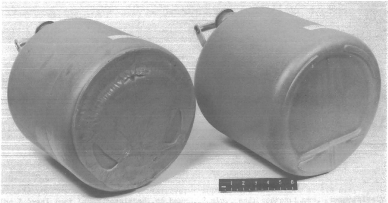
FIGURE 3. - Plastic safety container after 1/2-h contact with hot plate at 572° F (left) and a new container (right).
