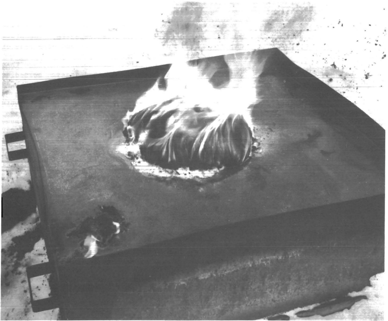
FIGURE 5. - Remnants of plastic pail and 35 lb of grease 8 min after tray fire has self-extinguished.
