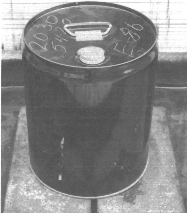
FIGURE 8. - Black metal container prior to standard tray fire test.
