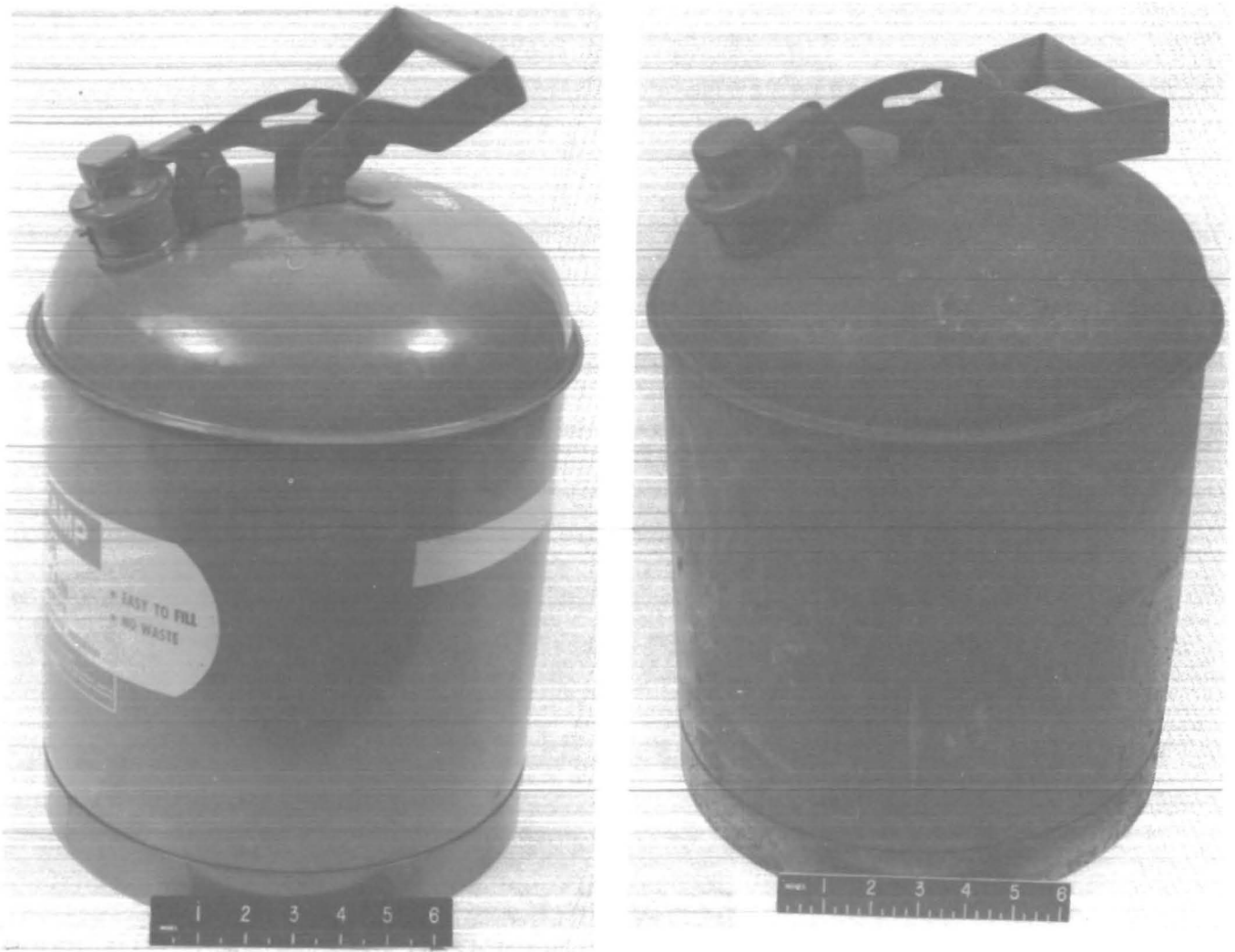
FIGURE A-15. - Metal safety containers before and after standard tray fire (NFR oil contents).
