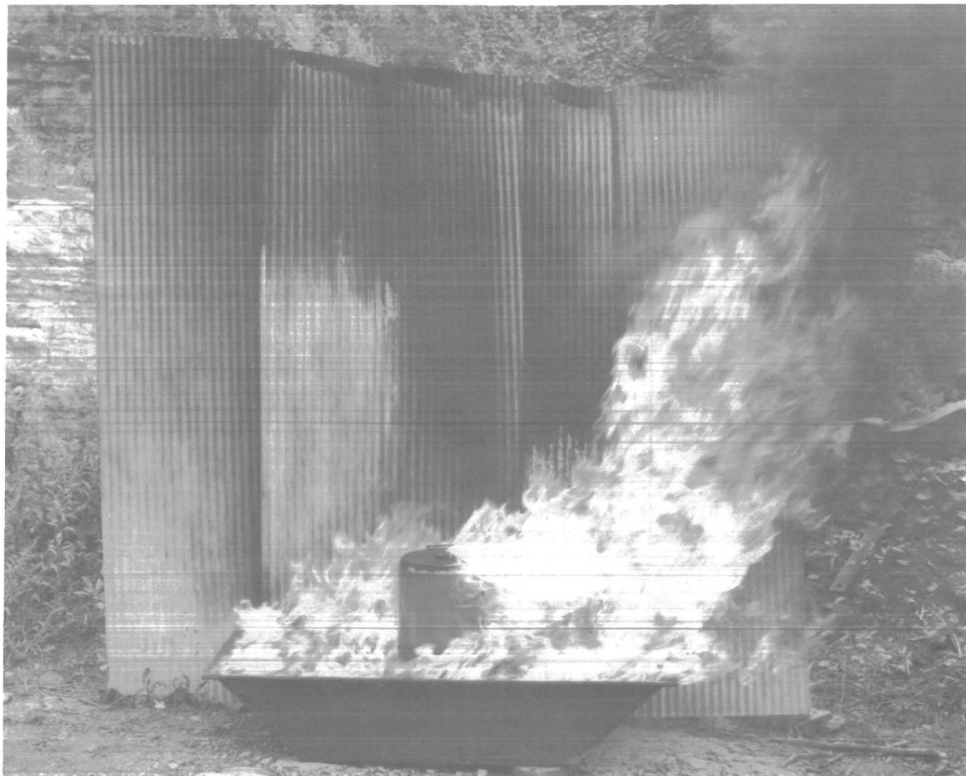
FIGURE 9. - Usual mode of pressure release from black container (flame jet near screw cap closure).
