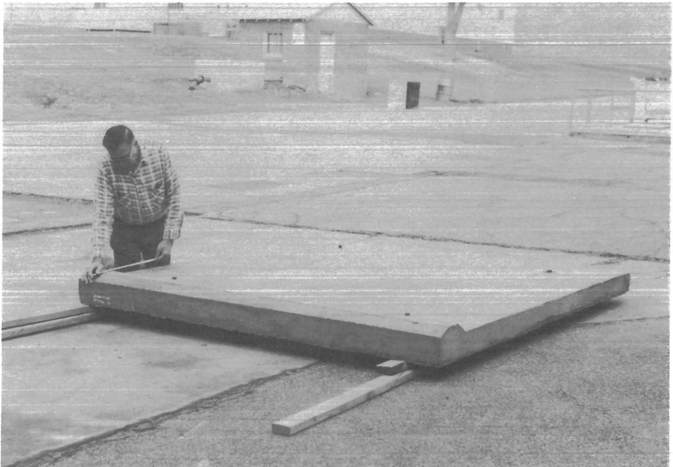
FIGURE 7. - A glass-fiber concrete pad for use in battery-dumping unit.
