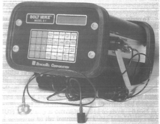
Figure 8.—Bolt Mike S-1 measurement device.
