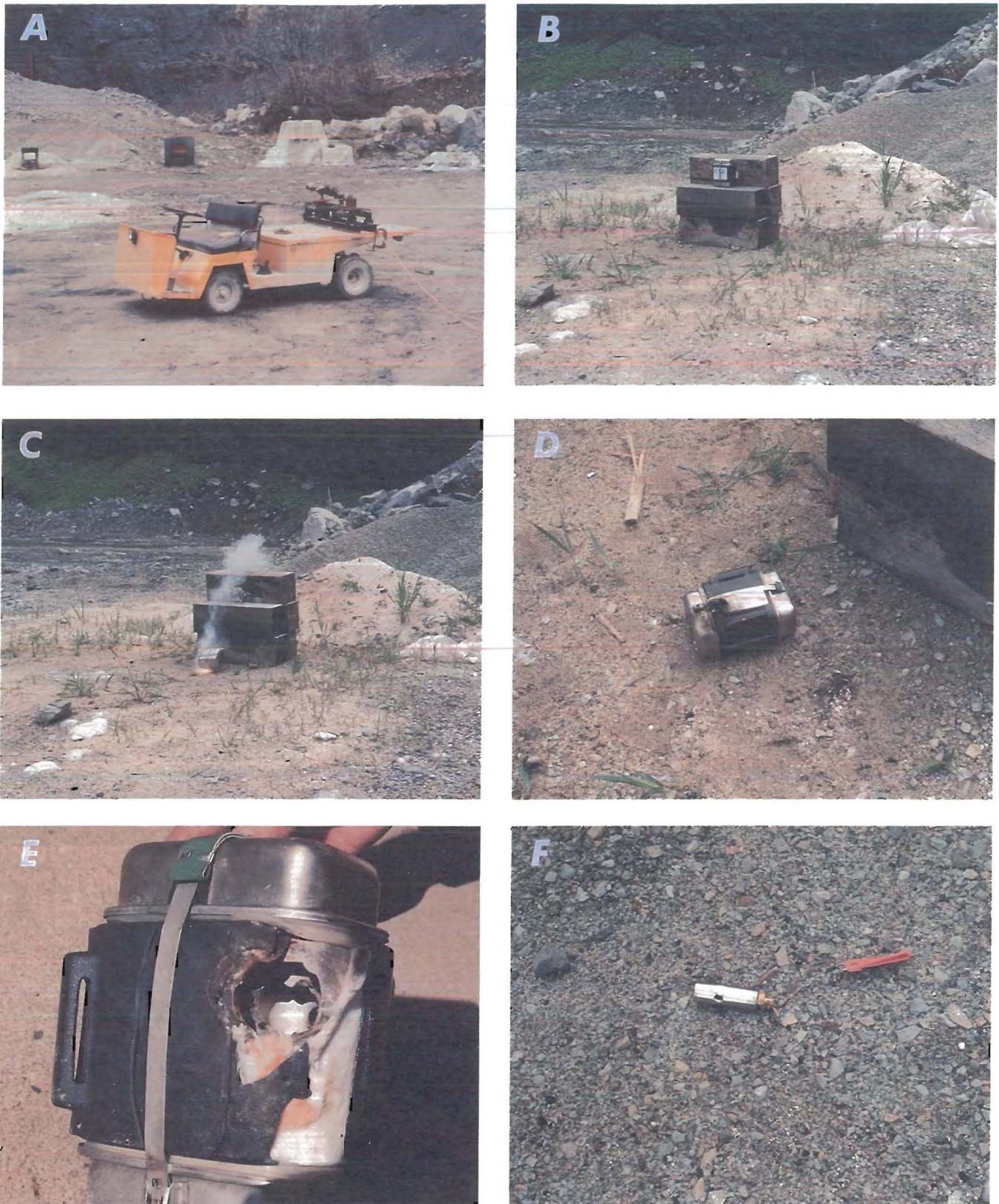
Figure 3.—Bullet Impact trials. A-B, Experimental setup; C, fire in test 4; D, exit hole in test 4; E, exit hole in test 2; F, oxygen bottle from test 5.
