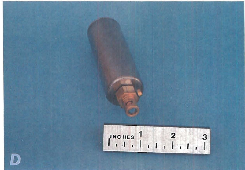
Figure 1.—Construction features of SR-100. A, Complete unit; B, unit ready for use; C, disassembled canister; D, oxygen bottle.
