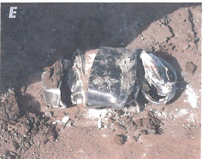
Figure 8.—Bulldozer runover trials. A , Unit perpendicular to direction of travel; B , unit parallel to direction of travel on coalbed; C , puff of smoke observed in test 2, run 1; D , total damage to unit in test 1; E , total damage to unit in test 2; F , total damage to unit in test 3.
