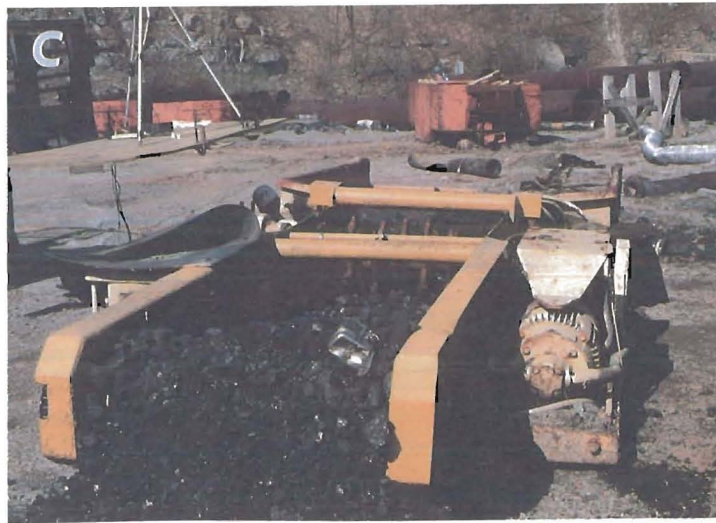
Figure 11.—Feeder-breaker trial with randomly placed units (test 1, run 1). A, Unit on coalbed; B, feeder-breaker running; C, unit being fed out of breaker.
