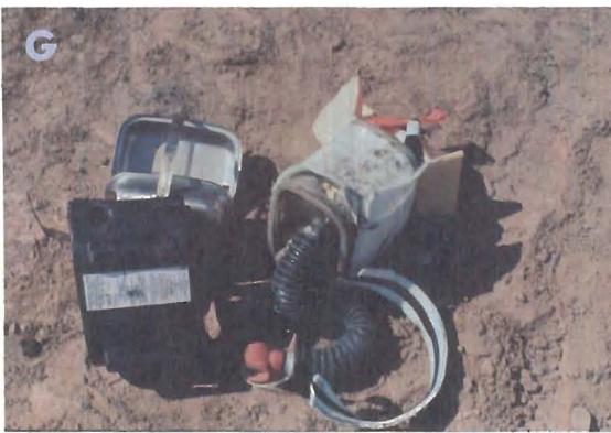
Figure 12.—Total damage to units used in feeder-breaker trials with randomly placed units. A-H, Tests 1 through 8, respectively.
