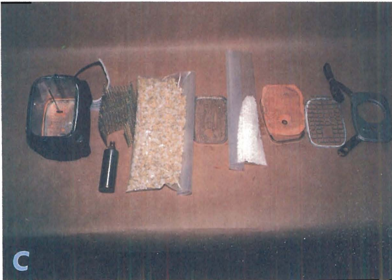
Figure 1.—Construction features of SR-100. A, Complete unit; B, unit ready for use; C, disassembled canister; D, oxygen bottle.
