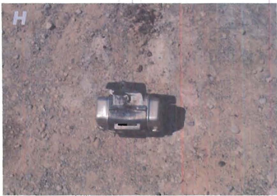
Figure 12.—Total damage to units used in feeder-breaker trials with randomly placed units. A-H, Tests 1 through 8, respectively.
