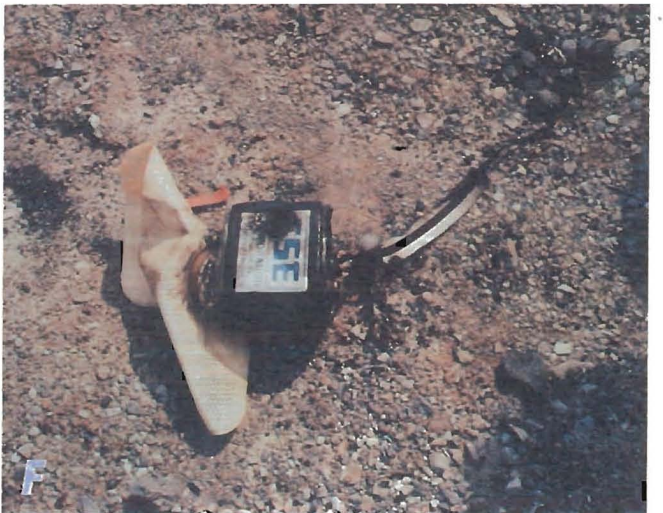
Figure 15.—Damage to units used in locked feeder-breaker trials. A-F, Tests 1 through 6, respectively.
