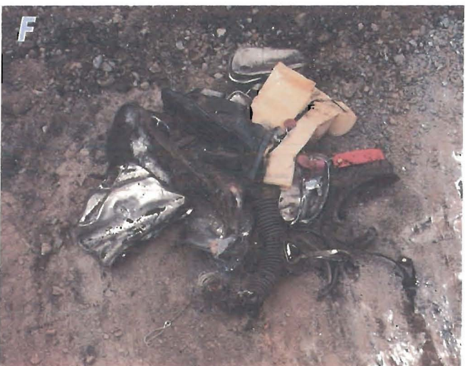
Figure 8.—Bulldozer runover trials. A , Unit perpendicular to direction of travel; B , unit parallel to direction of travel on coalbed; C , puff of smoke observed in test 2, run 1; D , total damage to unit in test 1; E , total damage to unit in test 2; F , total damage to unit in test 3.
