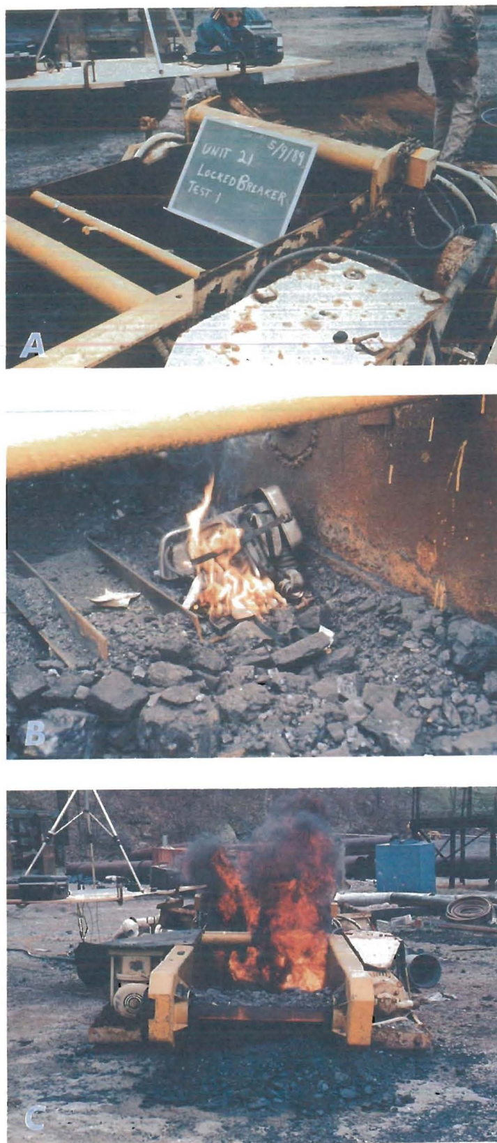
Figure 14.—Locked feeder-breaker trials. A, "Locked" feeder-breaker; B, fire observed in test 3; C, fireball observed in test 4.
