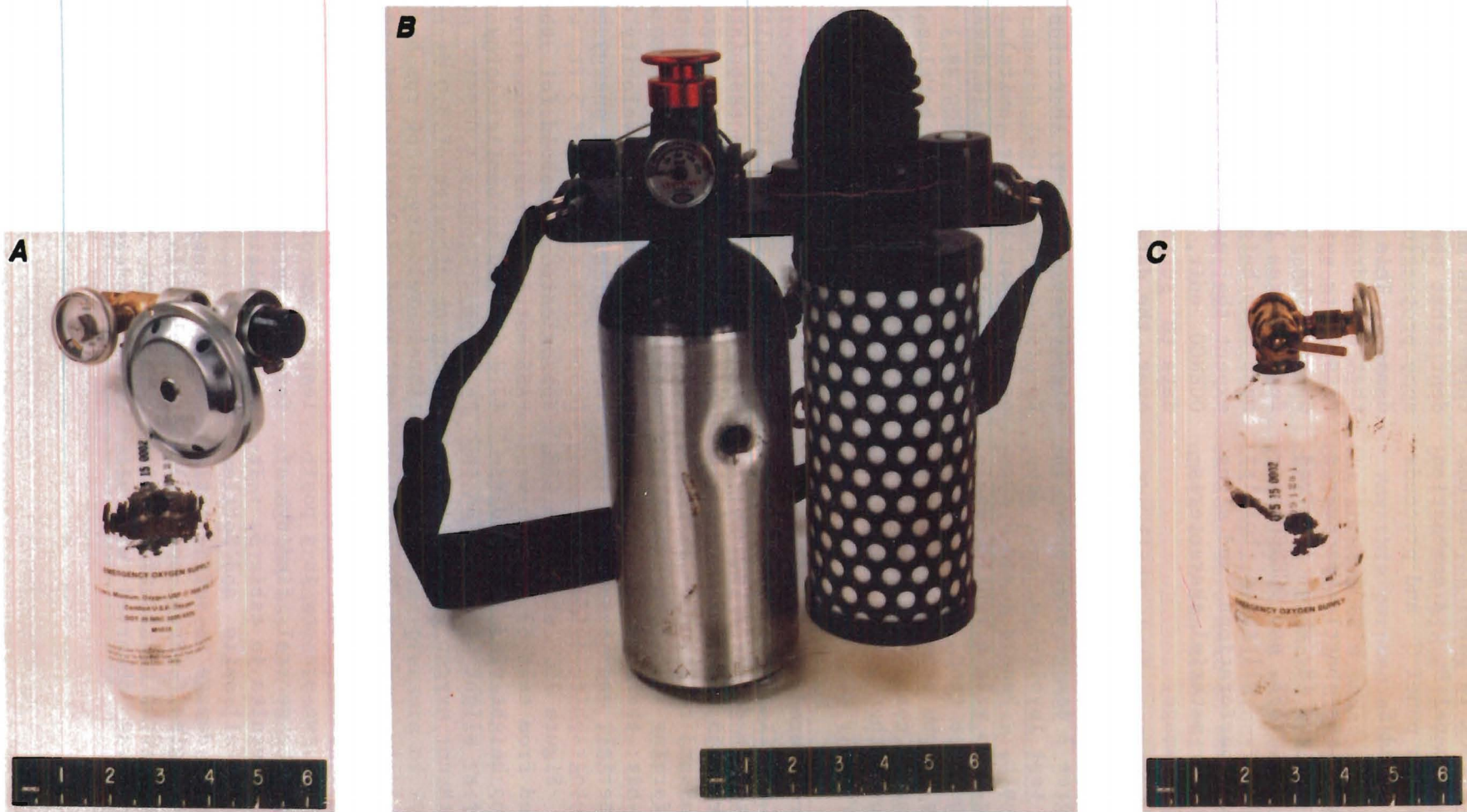
FIGURE 15. - Bottles recovered from drop weight tests (A) 94, (B) 148, and (C) 69, illustrating degree 2 damage (A-B) and degree 4 damage (C). The puncture holes did not display any excess size or discoloration associated with an impact induced combustion reaction.
