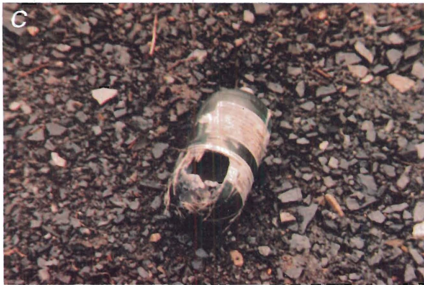
FIGURE 10. - Results of bullet impact tests. A , Still photograph of test 47 showing orange sparks and white cloud of aluminum oxide; B , CSE bottle from test 46; C , OCENCO bottle from test 47; D , PASS bottle from test 48.
