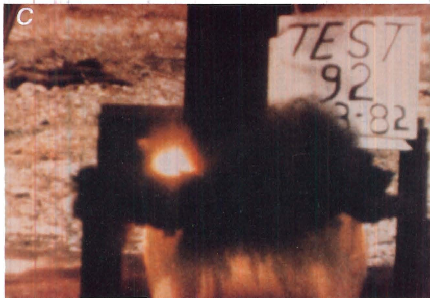
FIGURE 16. - Drop weight test 92 with a PASS unit showing ignition of added coal dust. The black cloud in panel B is coal dust dispersed at impact, which ignites in panels C and D .
