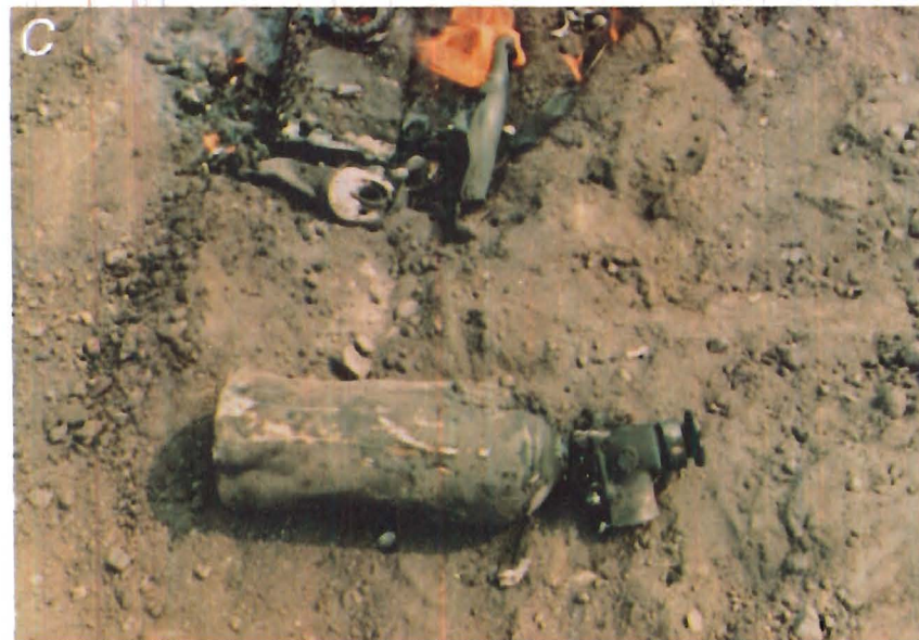
FIGURE 43. - Damage resulting from continuous miner runover trials. A , CSE bottle from test 162, degree 3; B , OCENCO bottle from test 163, degree 2; C , PASS unit from test 183, degree 1f (note orange flames on interior components); D , OCENCO unit from test 177, degree 1e (white entanglement is fiberglass overlay on bottle).
