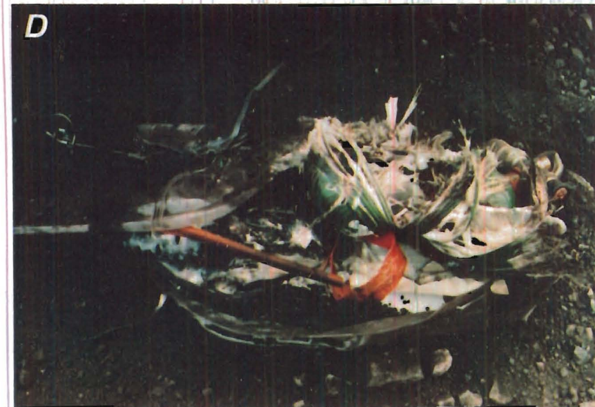
FIGURE 43. - Damage resulting from continuous miner runover trials. A , CSE bottle from test 162, degree 3; B , OCENCO bottle from test 163, degree 2; C , PASS unit from test 183, degree 1f (note orange flames on interior components); D , OCENCO unit from test 177, degree 1e (white entanglement is fiberglass overlay on bottle).
