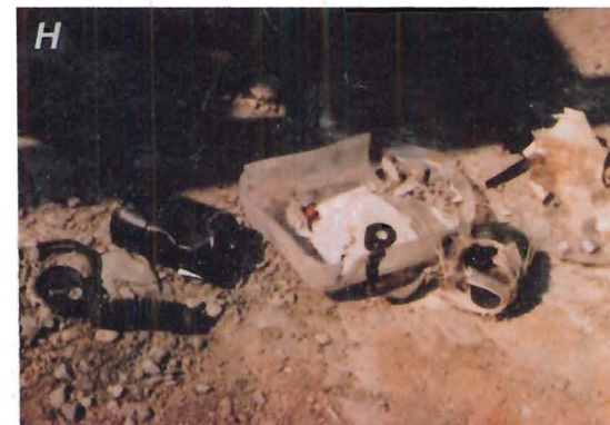
FIGURE 18. - Damage resulting from simulated roof falls with units in the flat position (A-C); units in the upright position (D-F); and units in the flat position with the rock shard (G-I). The rock shard which detached itself from the concrete block is embedded in the orange CSE case in panel G.
