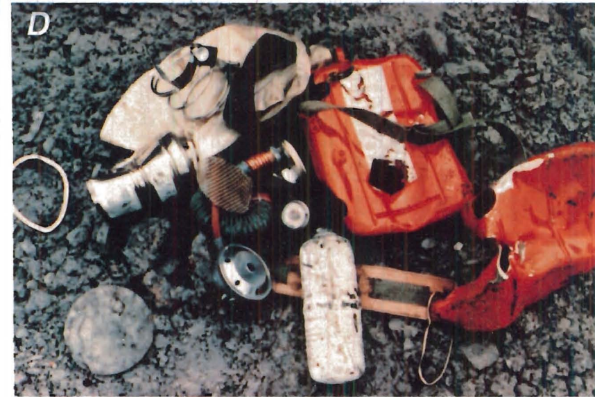
FIGURE 30. - Damage to units resulting from feeder-breaker impact. A , Flame-blackened bottle and interior components from test 97 with a CSE unit, degree 1e; B , punctured PASS bottle and damaged components from test 147, degree 2; C , damaged OCENCO bottle and components from test 135, degree 3; D , intact CSE bottle and other damaged components from test 142, degree 4.
