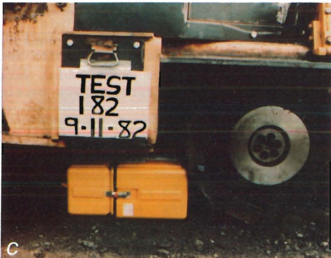
FIGURE 38. - A , Lee-Norse prototype miner; B , aluminum PASS bottle perpendicular to direction of travel; C , yellow PASS unit with bottle parallel to direction of travel.
