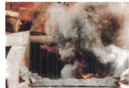
FIGURE 26. - Feeder-breaker impact test 97 with a CSE unit which resulted in damage of degree 1e. Flame from combustion reaction initiated in panel B completely engulfs interior of feeder-breaker.
