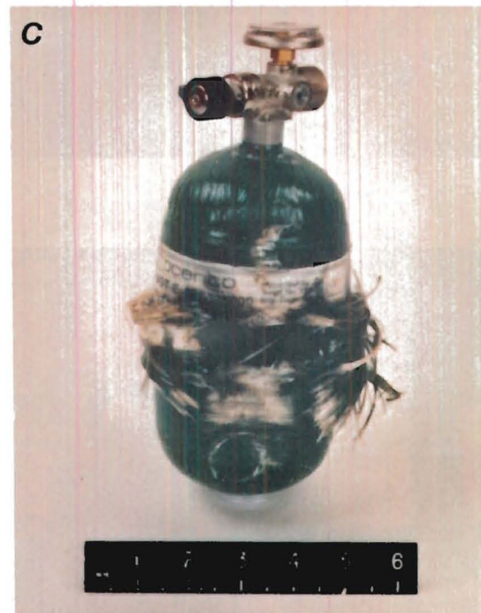
FIGURE 13. - Bottles recovered from tests (A) 20, (B) 34, and (C) 18, illustrating damage of degree 1e. Discoloration around perforations is characteristic of combustion reaction.
