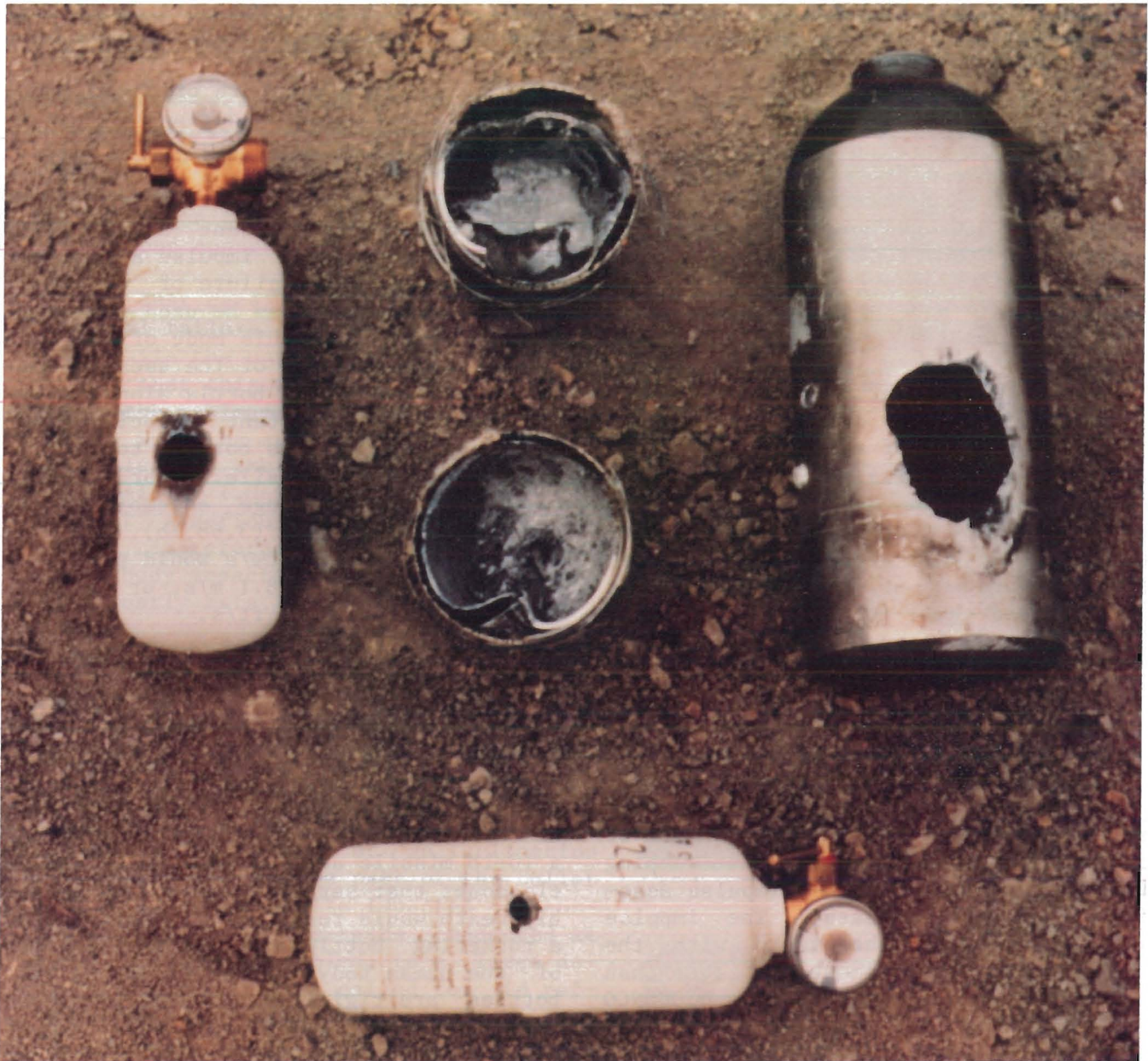
FIGURE 8. - Bullet impact damage to compressed oxygen bottles (top) compared with damage to bottle filled with compressed nitrogen (bottom). Grayish sludge in OCENCO bottle (top center) is molten aluminum.
