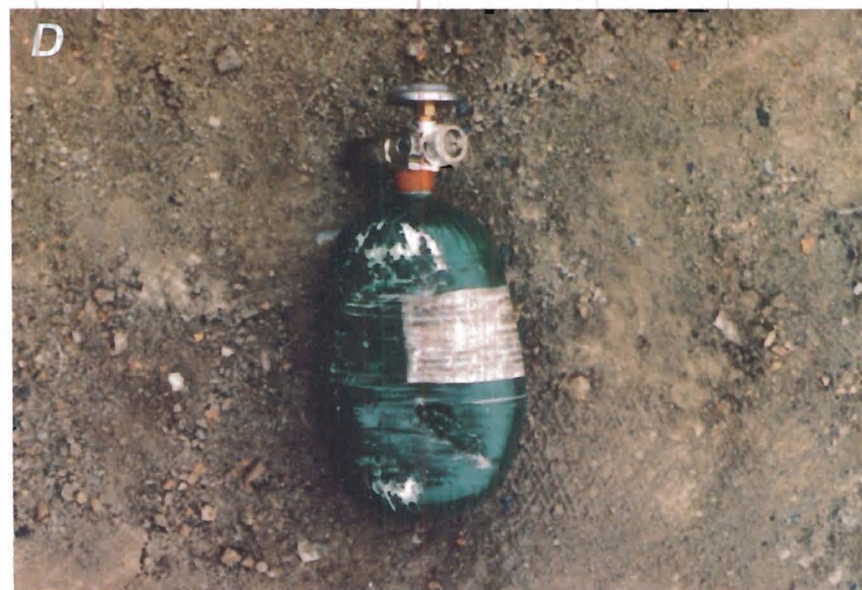
FIGURE 25. - Bottle damage resulting from feeder-breaker impacts. A , Flame-blackened OCENCO bottle from test 56, degree 1e; B , punctured PASS bottle from test 57, degree 2; C , CSE bottle with missing valve assembly, degree 3; D , dented but otherwise undamaged OCENCO bottle, degree 4.
