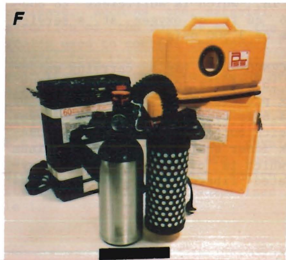
FIGURE 1. - The three self-rescuers used in test program. A-B , CSE; C-D , OCENCO; E-F , PASS. The orange exterior case of the CSE unit is of aluminum; the transparent case of the OCENCO unit and the yellow case of the PASS unit are plastic.
