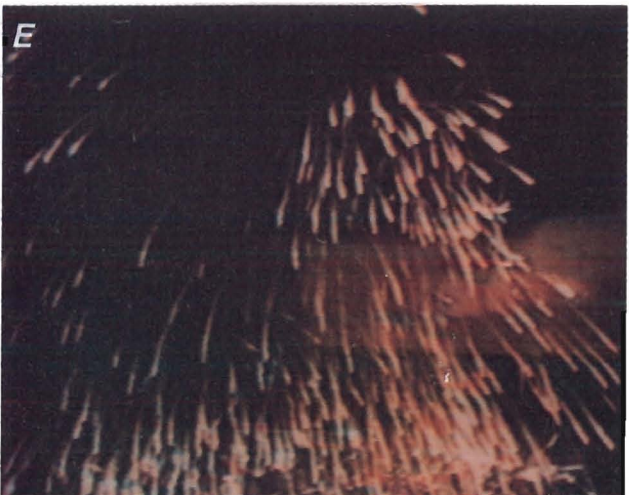
FIGURE 7. - Luminescent streamers associated with bullet impact on a CSE bottle in test 6.
