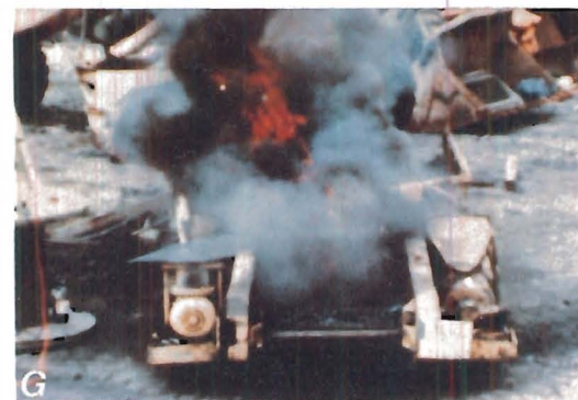
FIGURE 28. - Feeder-breaker impact test 186 with an OCENCO unit which resulted in damage of degree 1e. Intense white flame in panel B gradually fades to orangish-red in panel H.
