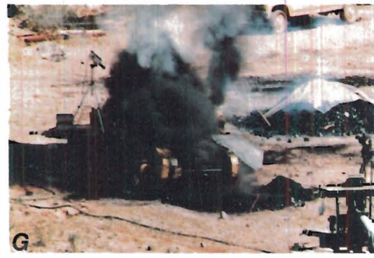
FIGURE 23. - Feeder-breaker impact test 64 with an OCENCO bottle which resulted in damage of degree 1e. Flame is clearly visible in panels C and D but is barely perceptible in panel E.
