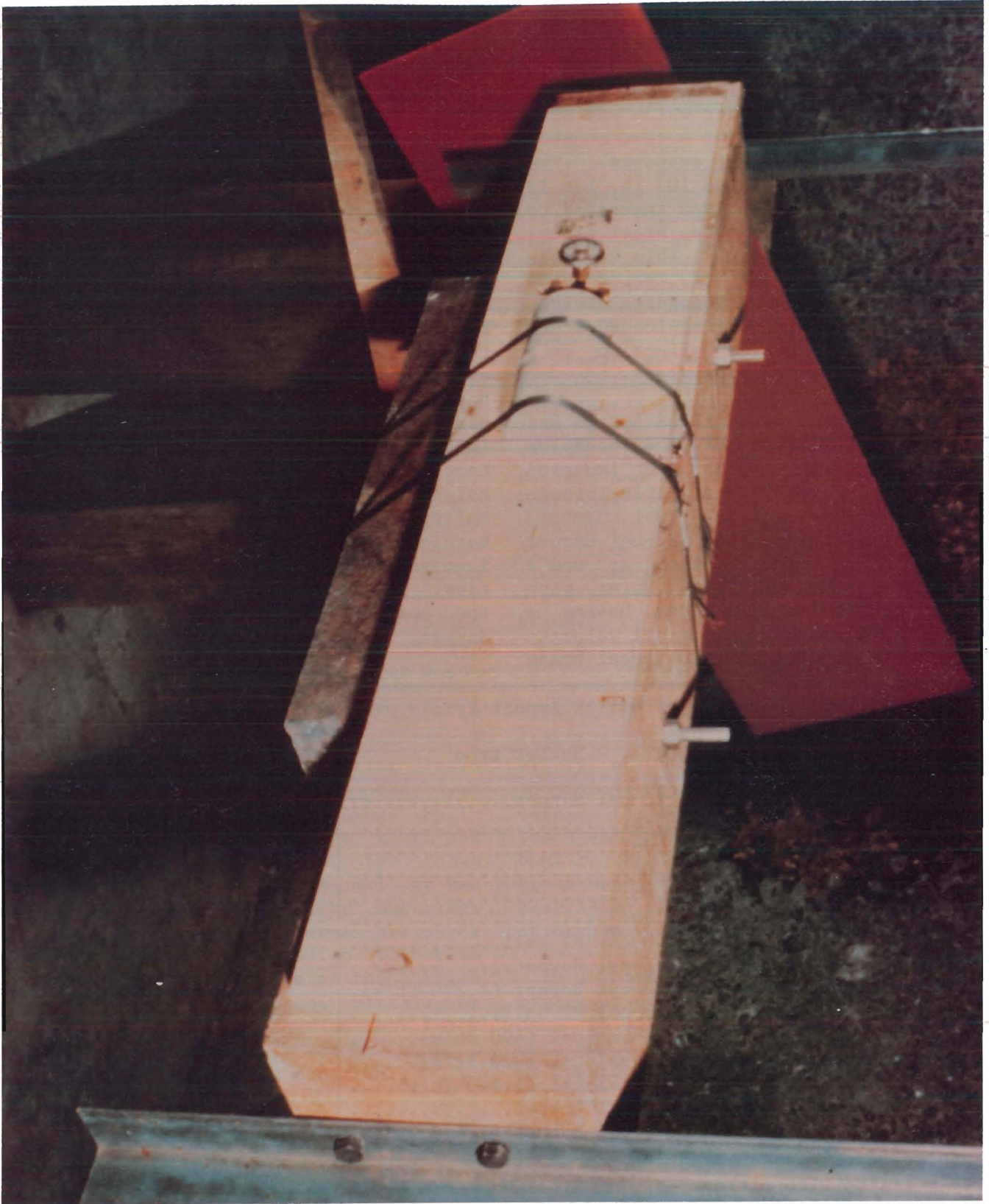
FIGURE 6. - Ballistic pendulum used to determine impulse associated with bottle puncture. White CSE bottle strapped to oak log is impacted by bullet traveling from left to right; red sheet in background is used to record pendulum deflection.
