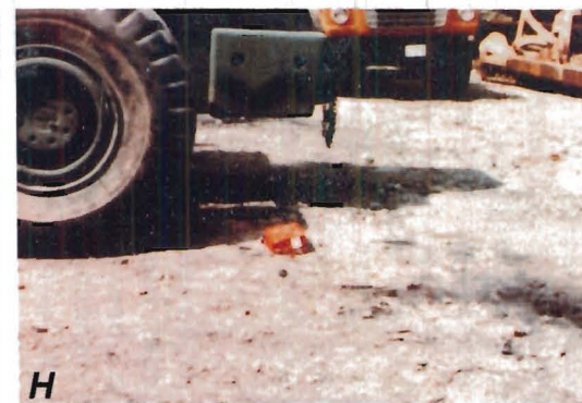
FIGURE 44. - Rubber-tired runover test 189 with an orange CSE unit which resulted in damage of degree 4.
