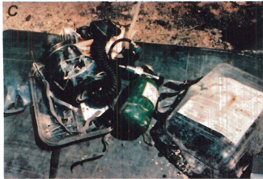
FIGURE 30. - Damage to units resulting from feeder-breaker impact. A , Flame-blackened bottle and interior components from test 97 with a CSE unit, degree 1e; B , punctured PASS bottle and damaged components from test 147, degree 2; C , damaged OCENCO bottle and components from test 135, degree 3; D , intact CSE bottle and other damaged components from test 142, degree 4.
