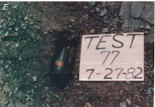
FIGURE 5. - Flame-blackened bottles recovered from bonfire tests 43, 44, and 45 (A-C) and remains of units recovered from tests 76, 77, and 78 (D-F).
