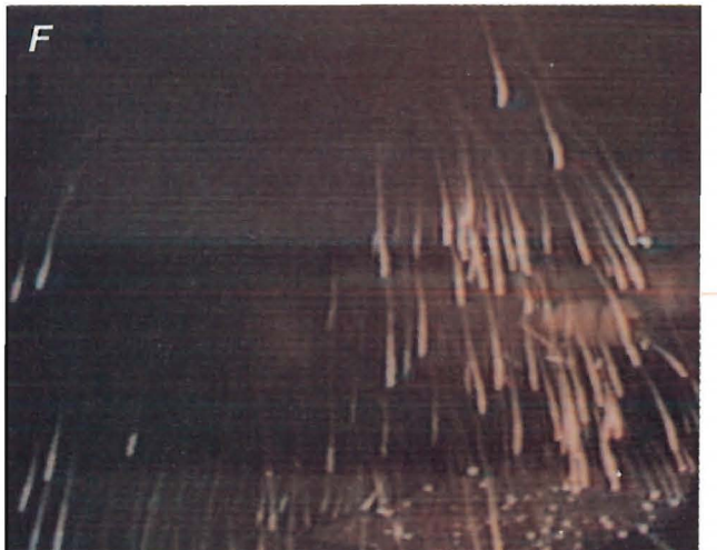
FIGURE 7. - Luminescent streamers associated with bullet impact on a CSE bottle in test 6.
