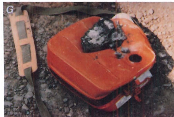
FIGURE 18. - Damage resulting from simulated roof falls with units in the flat position (A-C); units in the upright position (D-F); and units in the flat position with the rock shard (G-I). The rock shard which detached itself from the concrete block is embedded in the orange CSE case in panel G.
