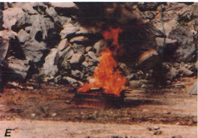
FIGURE 4. - Selected photographs from bonfire test 43 with a CSE bottle (A-B), test 44 with an OCENCO bottle (C-D), and test 45 with a PASS bottle (E-F). The large fireball in panel B and the intense white flames in panels D and F are associated with the rapid release of oxygen.
