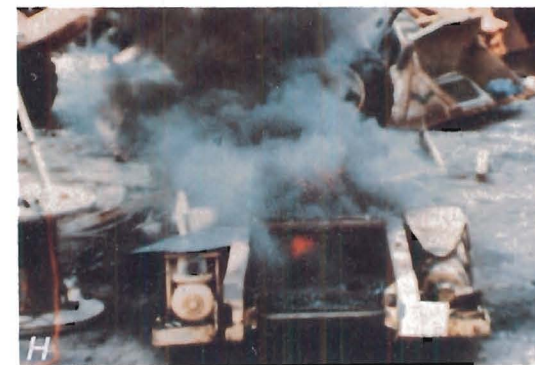
FIGURE 28. - Feeder-breaker impact test 186 with an OCENCO unit which resulted in damage of degree 1e. Intense white flame in panel B gradually fades to orangish-red in panel H.
