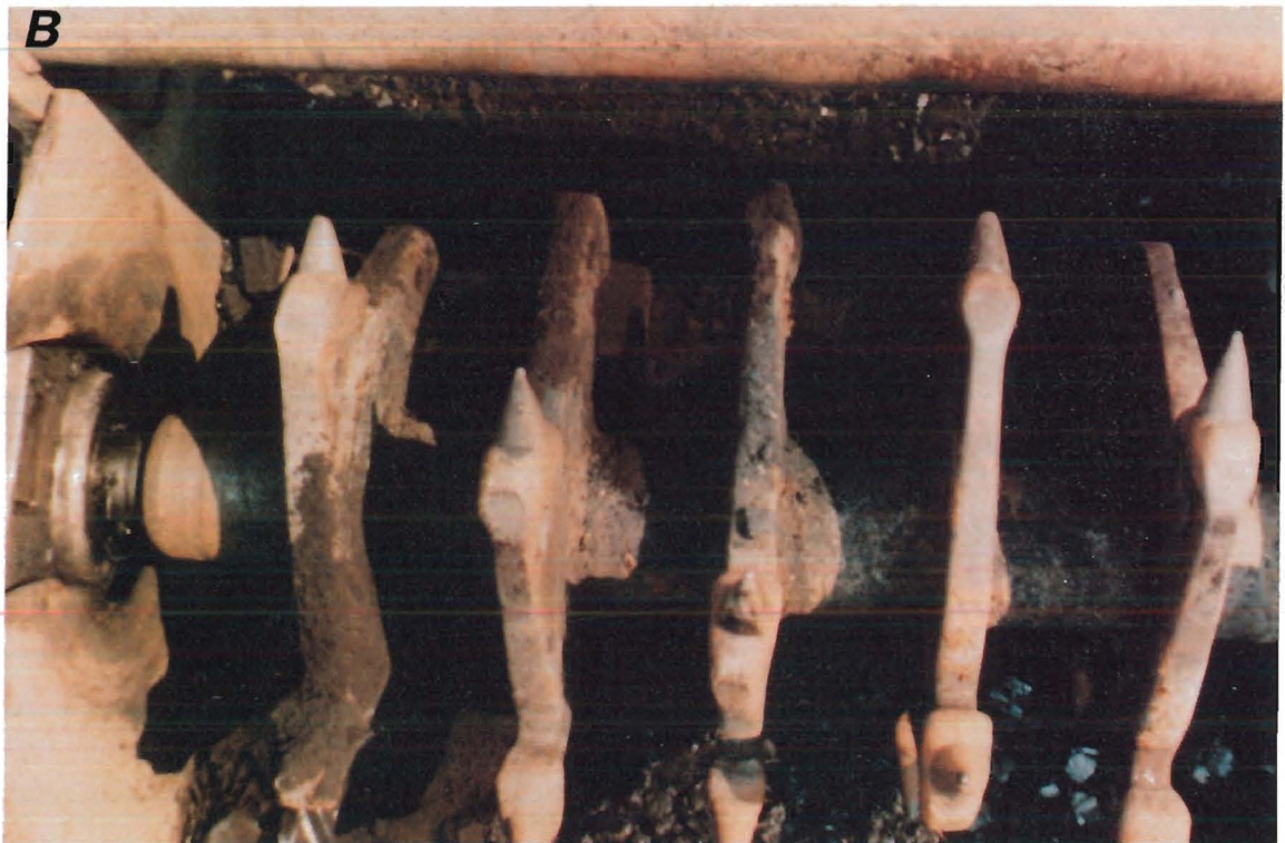
FIGURE 21. - A , Long-Airdox feeder-breaker; B , cutting head showing picks tipped with tungsten carbide.
