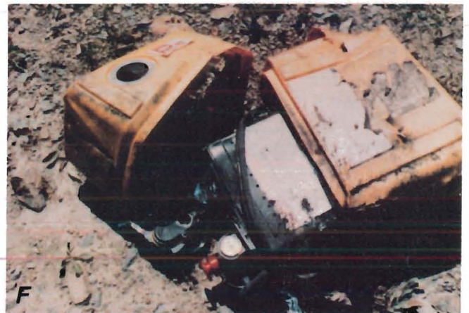
FIGURE 33. - Damage resulting from feeder-breaker feed-through trials. A , Test 132-1 with a CSE unit, degree 3; B , test 121 with a CSE unit, degree 4; C , test 129-1 with an OCENCO unit, degree 3; D , test 131 with an OCENCO unit, degree 4; E , test 123 with a PASS unit, degree 3; F , test 124 with a PASS unit, degree 4.
