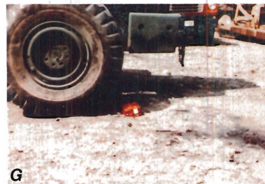
FIGURE 44. - Rubber-tired runover test 189 with an orange CSE unit which resulted in damage of degree 4.
