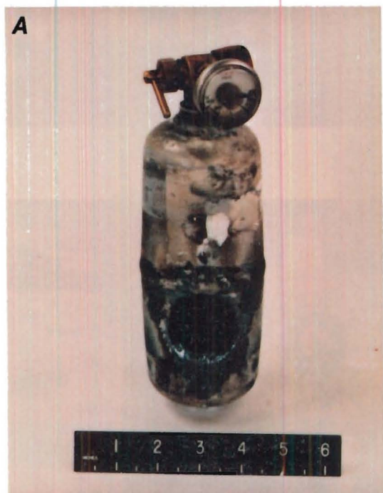
FIGURE 13. - Bottles recovered from tests (A) 20, (B) 34, and (C) 18, illustrating damage of degree 1e. Discoloration around perforations is characteristic of combustion reaction.
