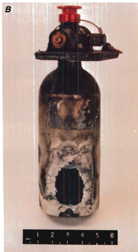
FIGURE 13. - Bottles recovered from tests (A) 20, (B) 34, and (C) 18, illustrating damage of degree 1e. Discoloration around perforations is characteristic of combustion reaction.
