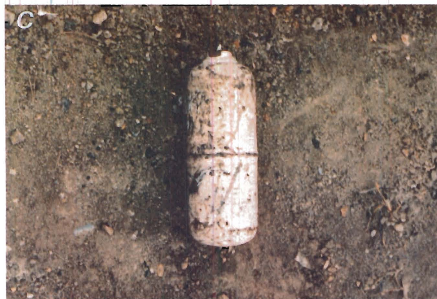
FIGURE 25. - Bottle damage resulting from feeder-breaker impacts. A , Flame-blackened OCENCO bottle from test 56, degree 1e; B , punctured PASS bottle from test 57, degree 2; C , CSE bottle with missing valve assembly, degree 3; D , dented but otherwise undamaged OCENCO bottle, degree 4.
