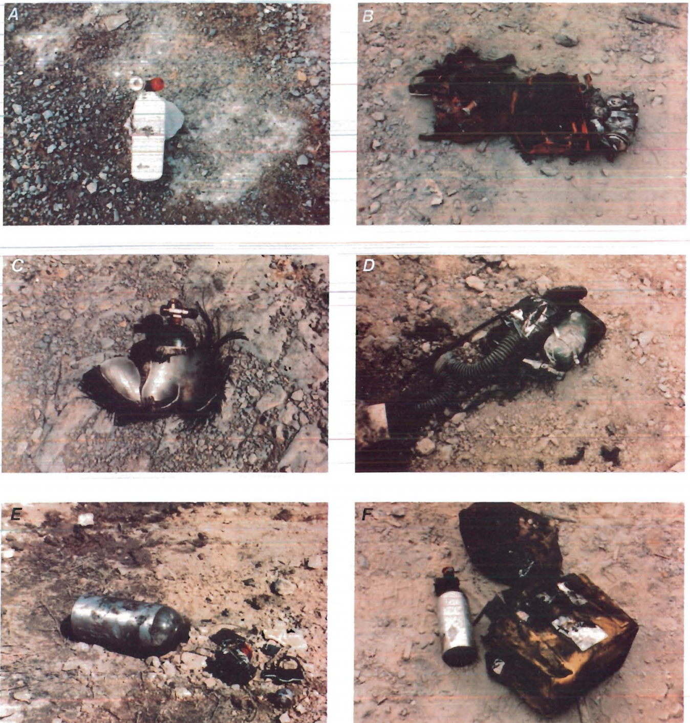
FIGURE 37. - Remnants of bottles and units from feeder-breaker runover trials. A , White CSE bottle from test 61, degree 3; B , CSE unit blackened with coal dust from test 73, degree 3; C , OCENCO bottle blown open in test 63, degree 1e; D , OCENCO unit blackened with coal dust from test 72, degree 3; E , damaged PASS bottle from test 62-1, degree 3; F , damaged PASS unit from test 71, degree 4.
