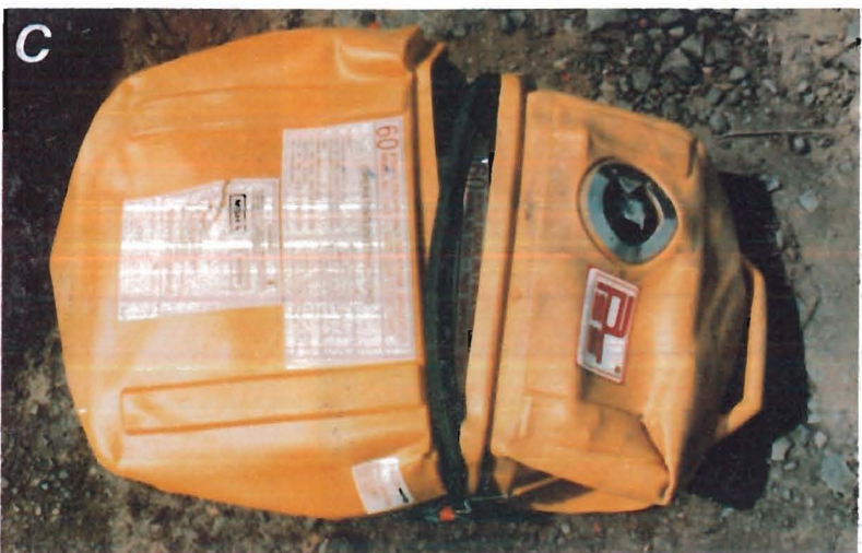
FIGURE 45. - SCSR's after having been repeatedly run over with a 30,000-lb rubber-tired vehicle. A , Orange CSE unit; B , transparent OCENCO unit; C , yellow PASS unit.
