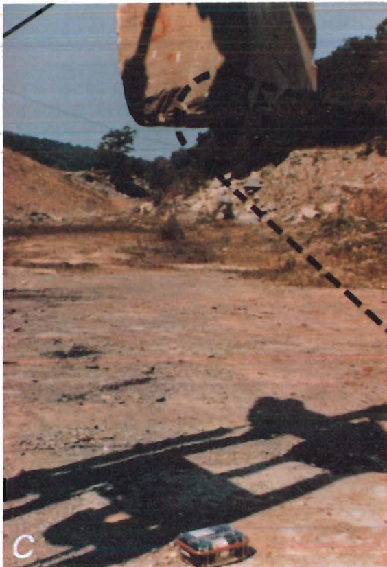
FIGURE 17. - Test configurations used in simulated roof fall trials. The dark brown rock shard in panel D was affixed to the bottom of the block in panel C with roof bolt resin.
