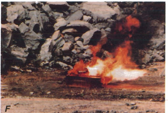
FIGURE 4. - Selected photographs from bonfire test 43 with a CSE bottle (A-B), test 44 with an OCENCO bottle (C-D), and test 45 with a PASS bottle (E-F). The large fireball in panel B and the intense white flames in panels D and F are associated with the rapid release of oxygen.
