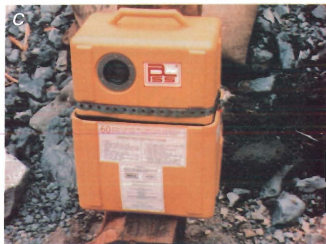
FIGURE 9. - Experimental setup used in outdoor bullet impact tests. A, Rifle mount and velocity station; B, bottle mounted at 45^\circ ; C, unit mounted for normal impact.
