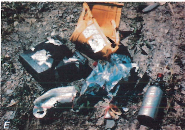
FIGURE 33. - Damage resulting from feeder-breaker feed-through trials. A , Test 132-1 with a CSE unit, degree 3; B , test 121 with a CSE unit, degree 4; C , test 129-1 with an OCENCO unit, degree 3; D , test 131 with an OCENCO unit, degree 4; E , test 123 with a PASS unit, degree 3; F , test 124 with a PASS unit, degree 4.
