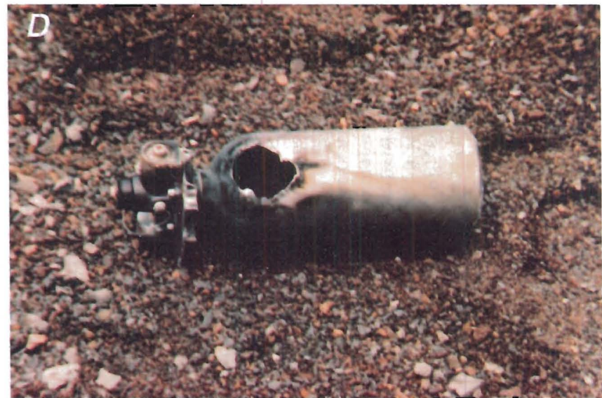
FIGURE 10. - Results of bullet impact tests. A , Still photograph of test 47 showing orange sparks and white cloud of aluminum oxide; B , CSE bottle from test 46; C , OCENCO bottle from test 47; D , PASS bottle from test 48.
