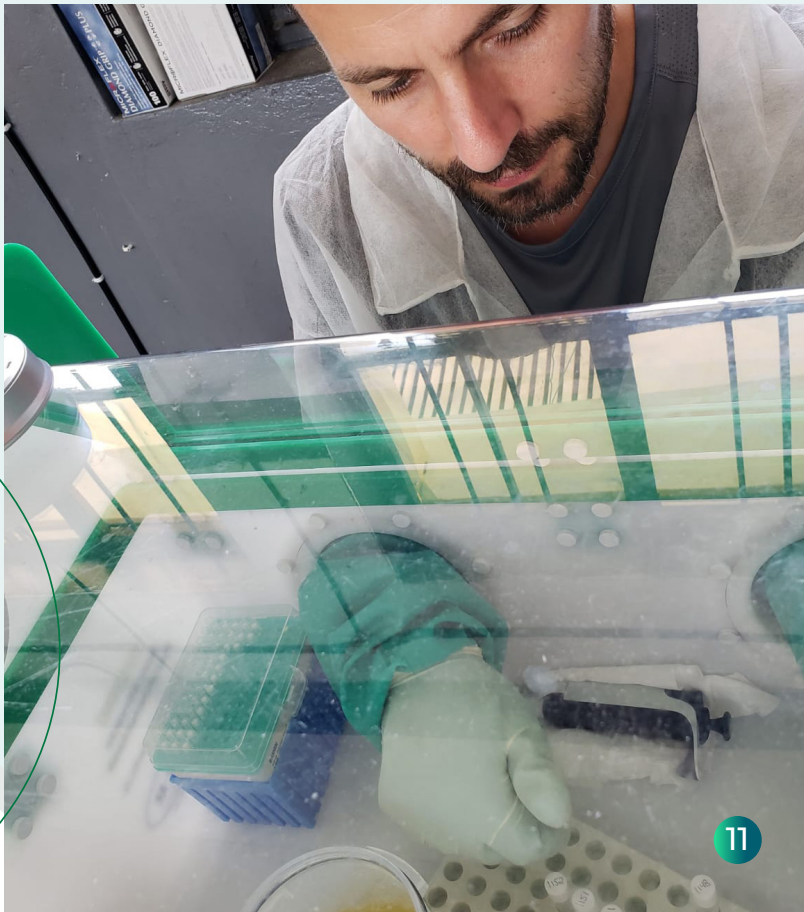
James Graziano using a piece of lab equipment called a “glove box” that CDC flew to DRC for use in the Ebola outbreak response. The glove box allows experts to safely work with patient samples while testing for Ebola.
