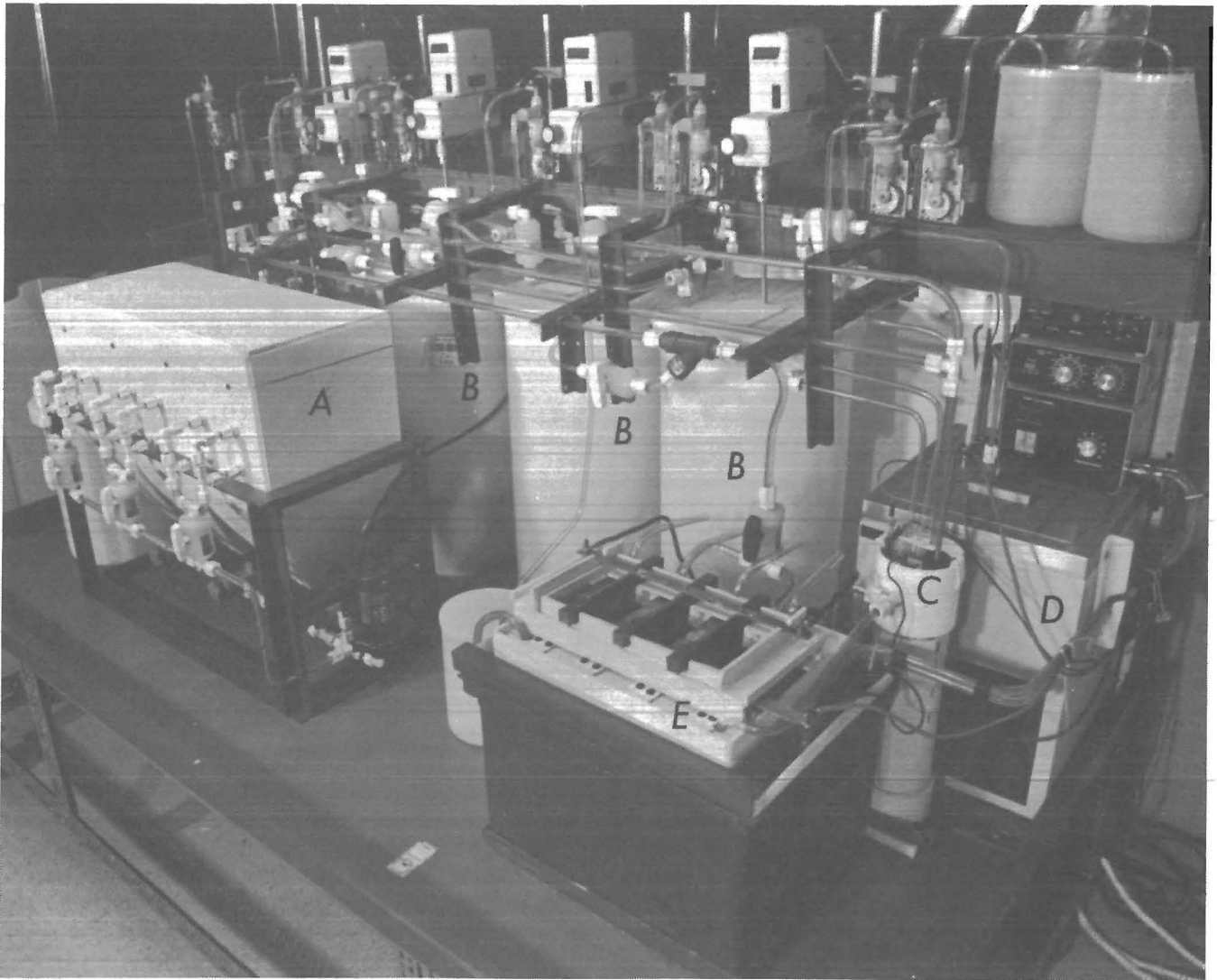
FIGURE 6. - Electrorefining unit. A , Anode wash tank; B , electrolyte storage tanks; C , auxiliary cell for monitoring polarization voltage; D , constant-temperature water bath; E , 20-L multi-electrode cell.
