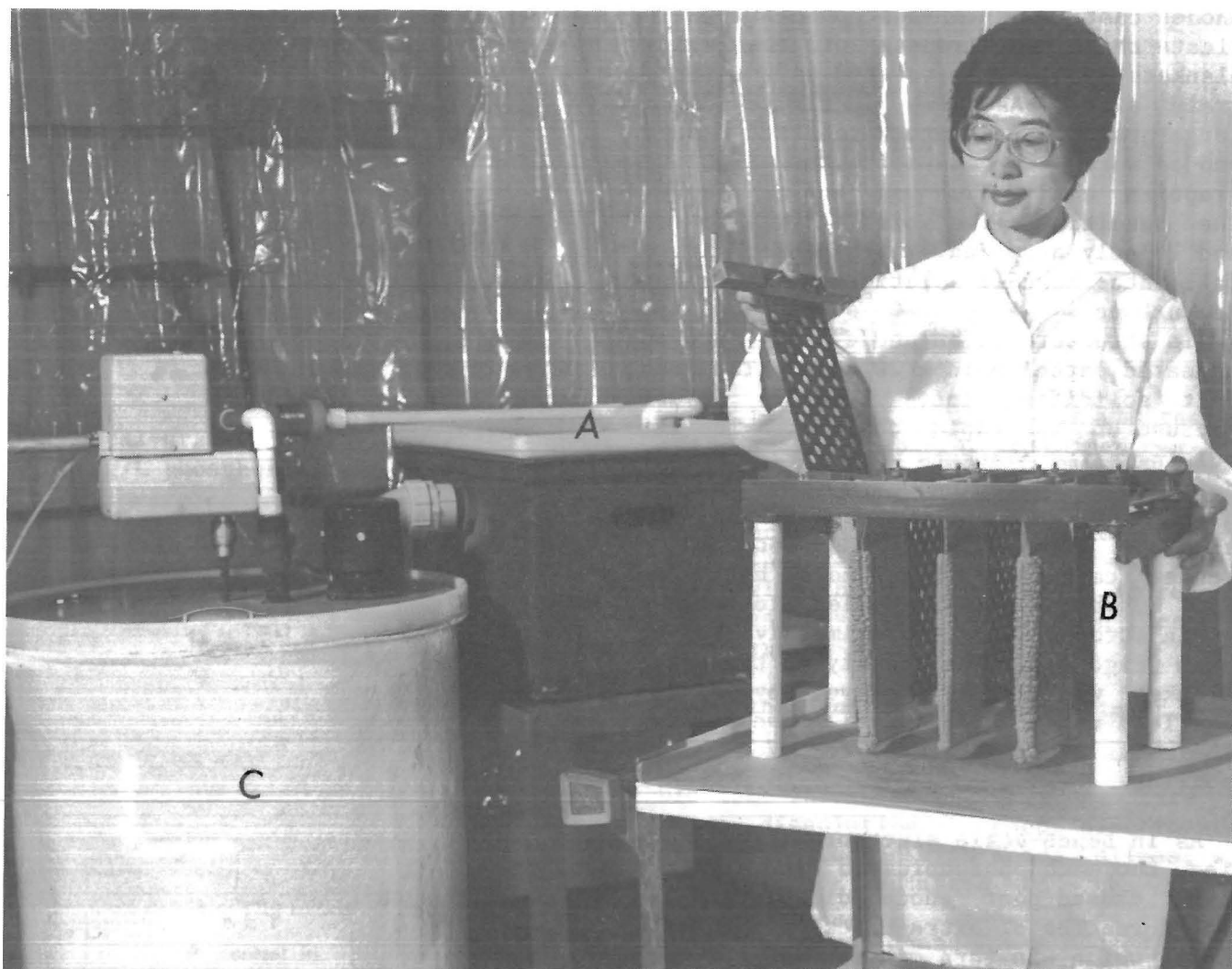
FIGURE 7. - Electrowinning unit. A , 20-L multielectrode cell; B , electrodes after a 5-day test; C , 200-L electrolyte tank.
