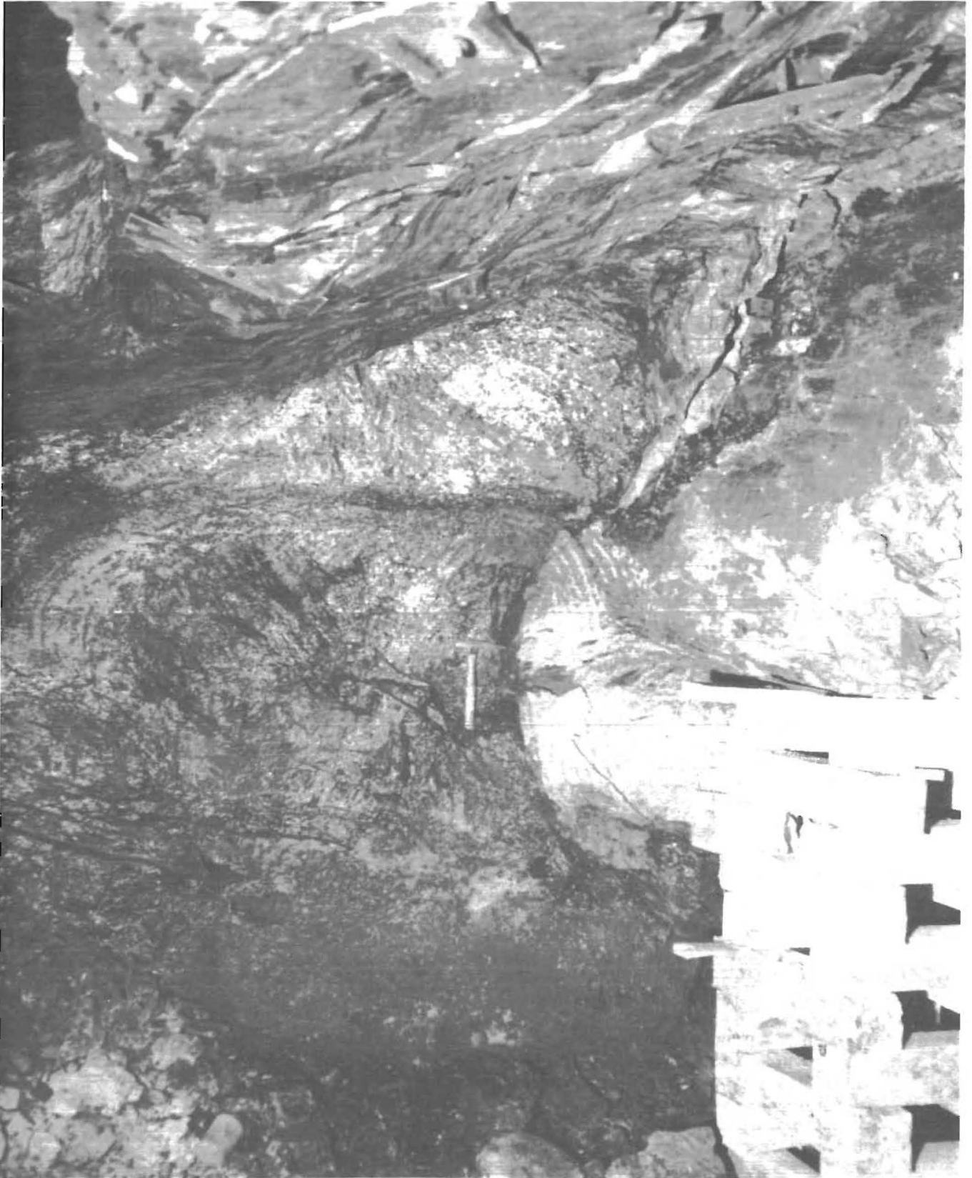
Figure 14.—Jawbone Coalbed split by compression along Pistol Gap Fault, with top half riding up into roof and bottom half pushed into floor.
