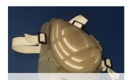
NIOSH prototype design of an EHMR with exhalation valves that filter exhaled breath. Photo by NIOSH
