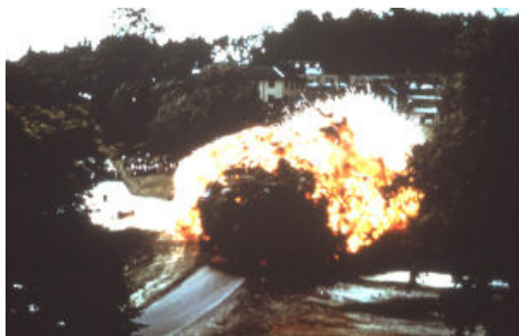
Test in the Experimental Mine studying the initiation and growth of coal dust explosions
