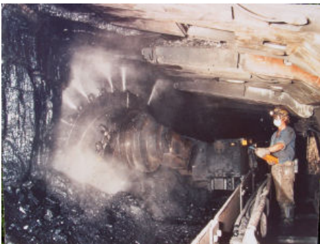
Water sprays on a longwall shearer to reduce respirable dust
