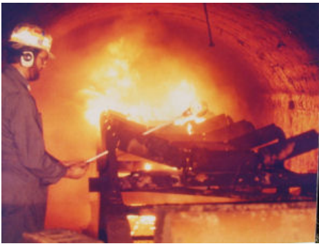
Test studying the behavior of fires along a mine conveyor belt
