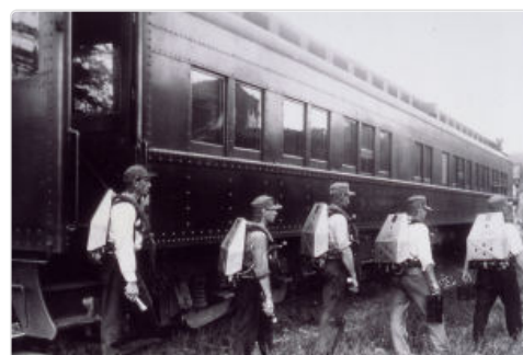
A Bureau of Mines mine safety railroad car equipped as a movable safety and rescue station.
