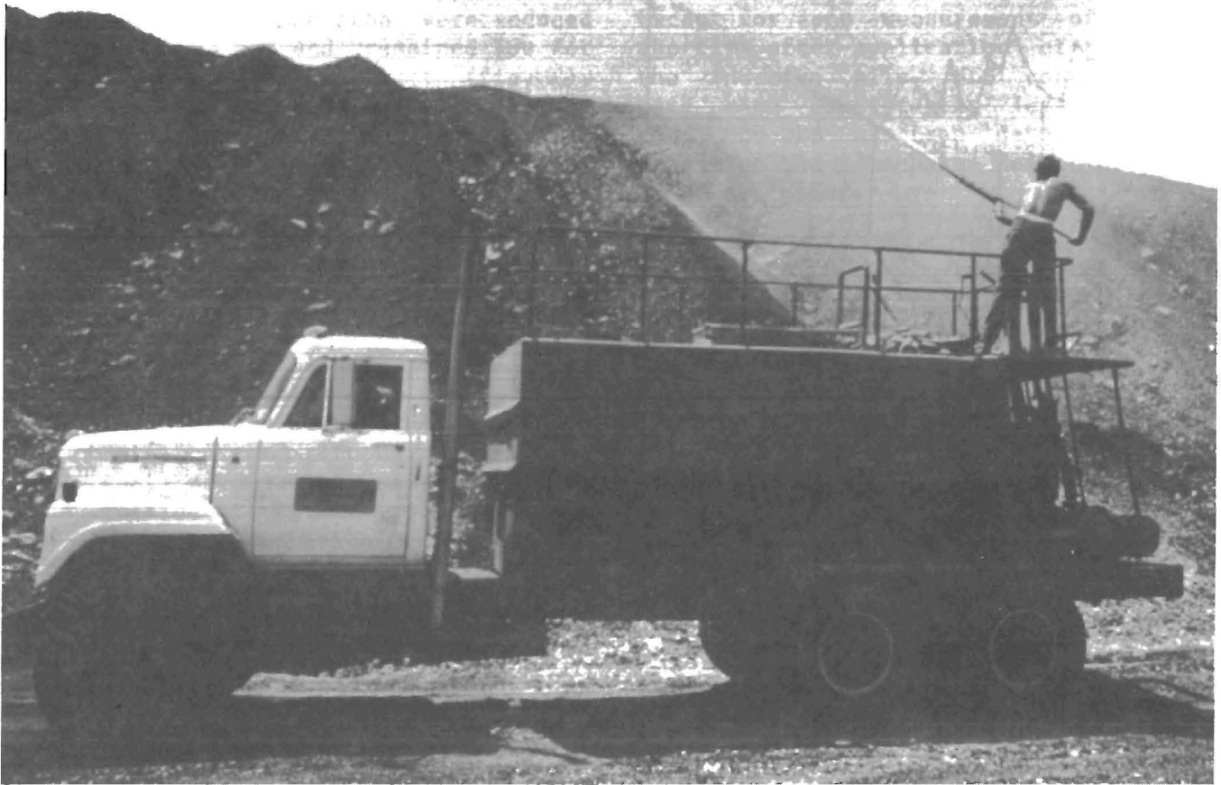
FIGURE 3. - Hydroseeder being used to spray sodium lauryl sulfate on 11-acre refuse area in southern West Virginia. Application rate: 55 gal/acre of 30-pct solution, diluted 175:1.
