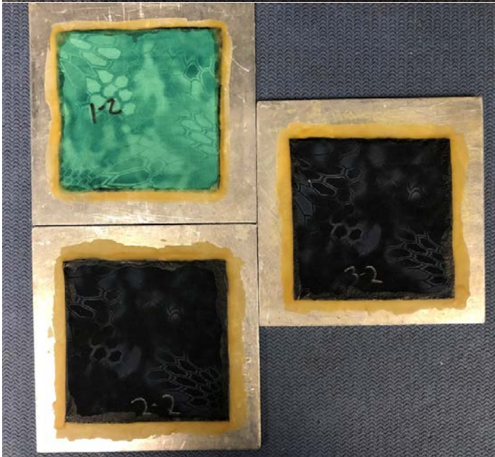
Figure S4: Samples fastened to test plate with beeswax in preparation for test of filtration efficiency and airflow resistance. A) Excellent Artisan procedure mask; B) BYD N95 respirator; C) AXBXCX neck gaiter.
