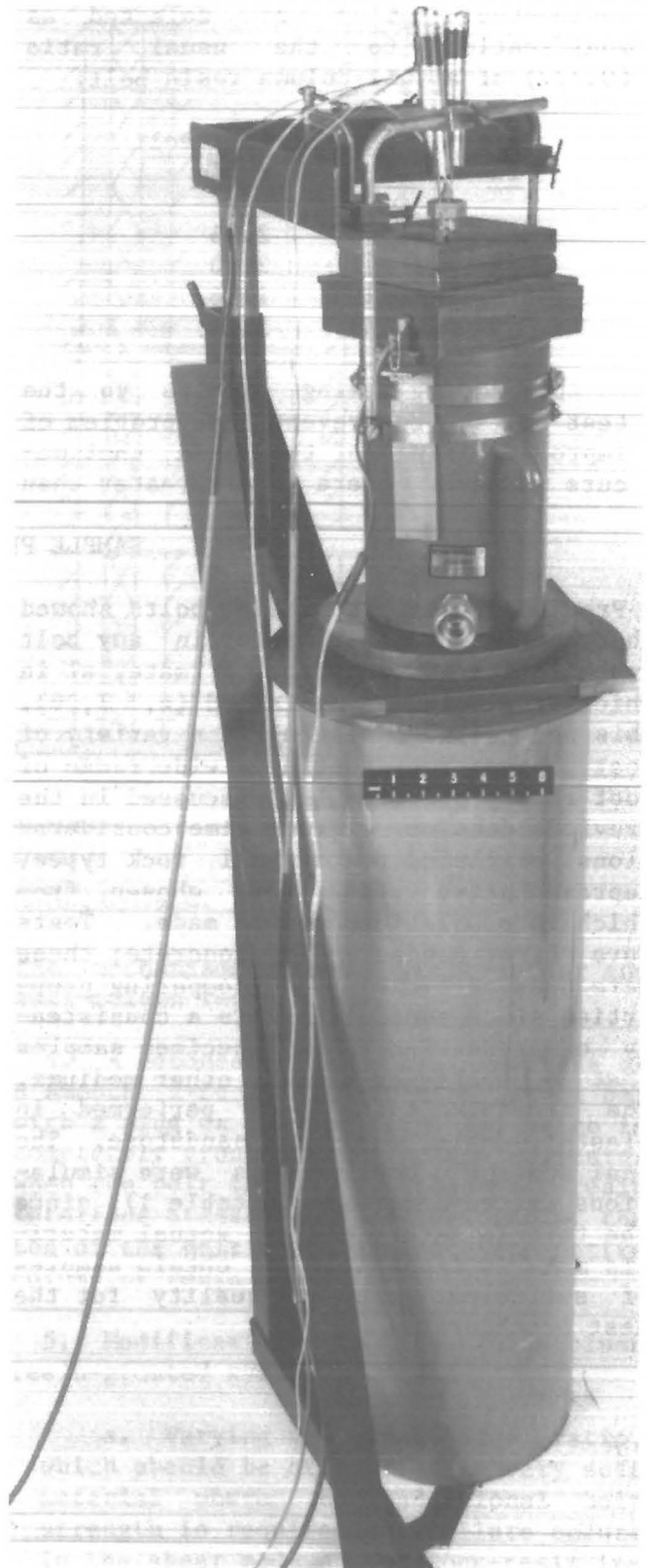
FIGURE 2. - Axial tension test setup.
