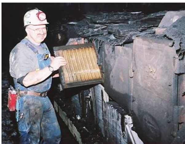
Fig. 7. Miner removing filter from scrubber (left) and graph showing respirable dust reductions with different density filters (right) (source: NIOSH)
