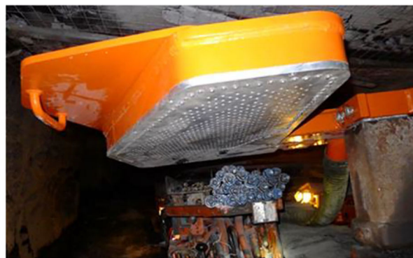
Fig. 9. Canopy air curtain provides filtered air to operator (left) and commercially available unit (right)
