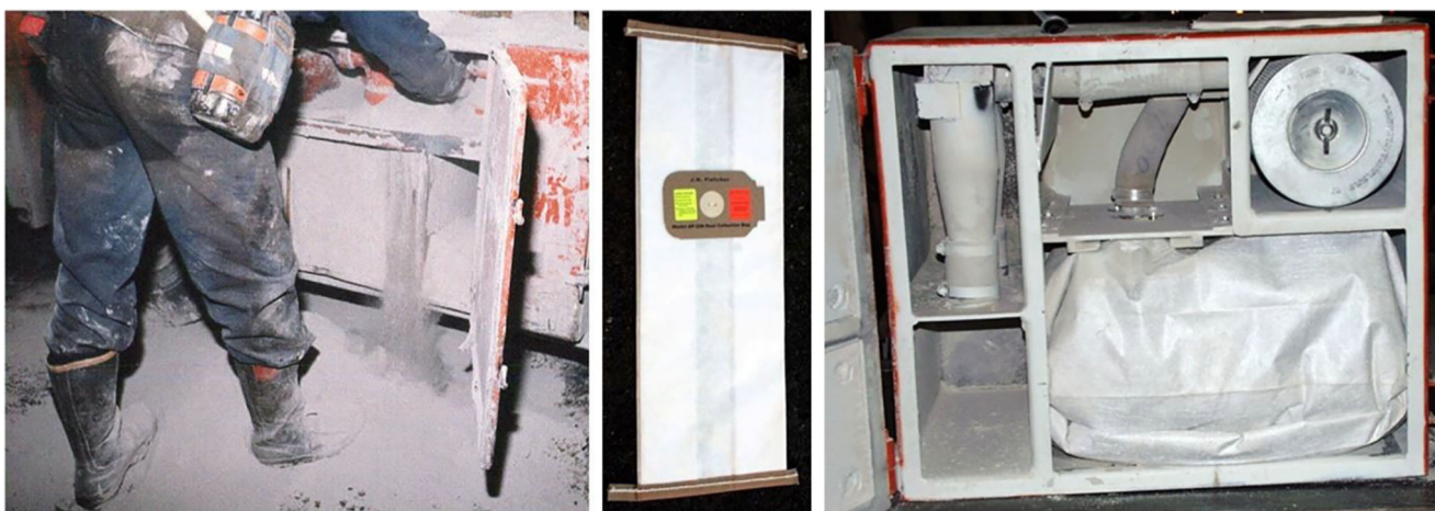
Fig. 8. Cleaning dust from collector box (left), collector bag (center), and dust captured in bag (right)
