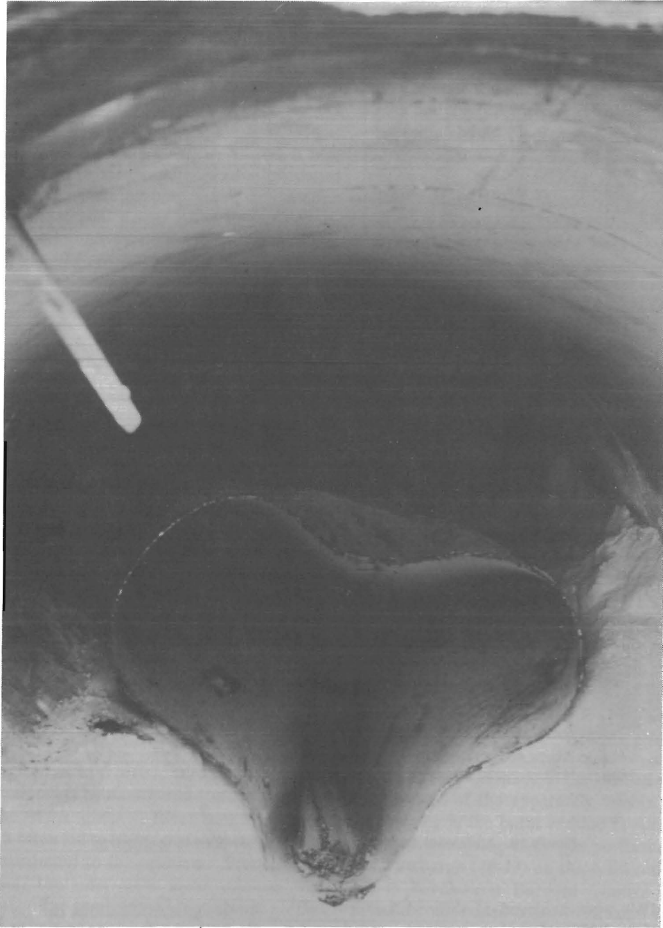
Figure 18.—Manifold cross section at position 15 ft into waste bank (during disassembly of system).
