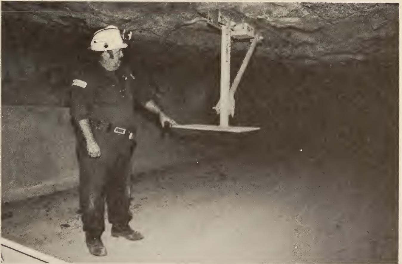
FIGURE 28. - Instrument platform that retracts into the roof of the entries—there are 38 such platforms installed in the facility.
