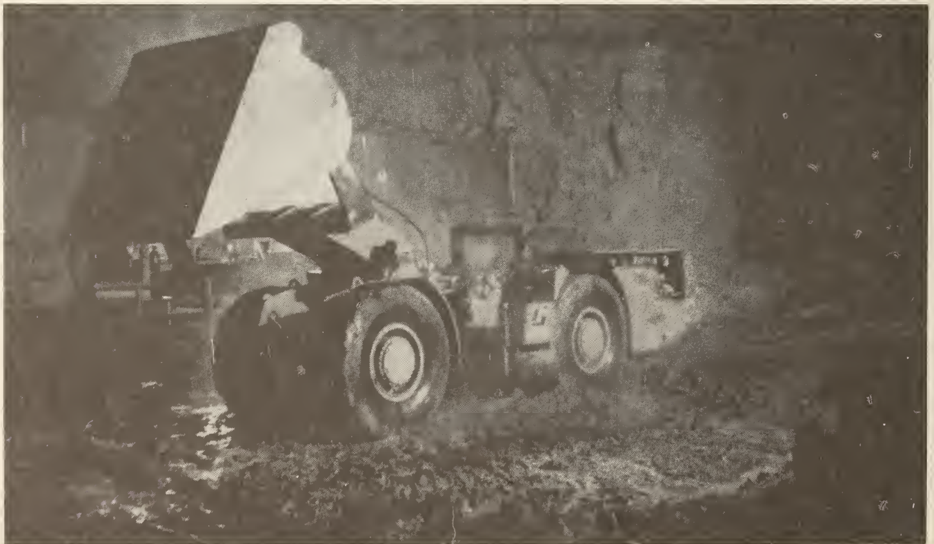
FIGURE A-11. - S.T.3 mucking buggy—used in transporting blasted limestone material out of the drifts.
