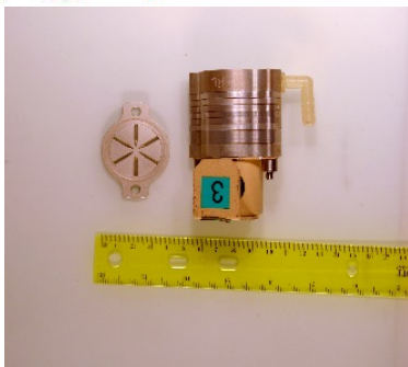
Figure 2J. Personal cascade impactor sampler (model Marple 290, Thermo Fisher Scientific). The sampler has five stages in the version shown and an additional three stages are available to provide cutpoints from 0.4 µm to 21 µm. The flap over the inlet reduces direct projection of large particles into the inlet. This sampler allows measurement of aerosol size distribution and calculation of respirable and thoracic fractions. It is constructed of aluminum and operates at 1.7 L/min.
