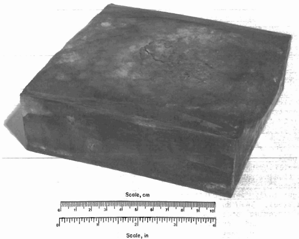
FIGURE 6. - Flaking of a test block. Mild steel (block 1) after 50,000 impacts.
