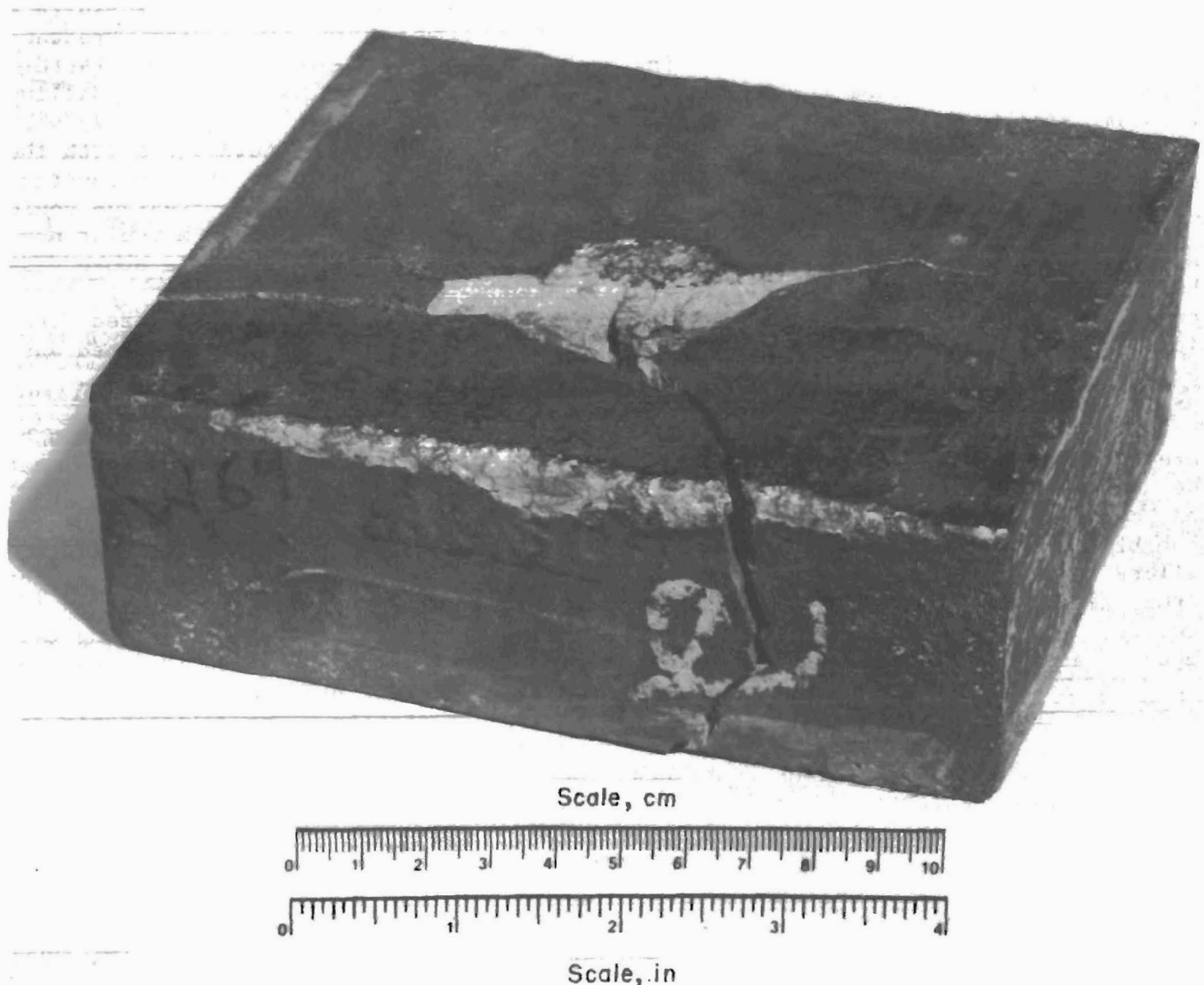
FIGURE 10. - Breakage of a test block. High Cr-Mo white cast iron (block 12c) after 40,300 impacts.
