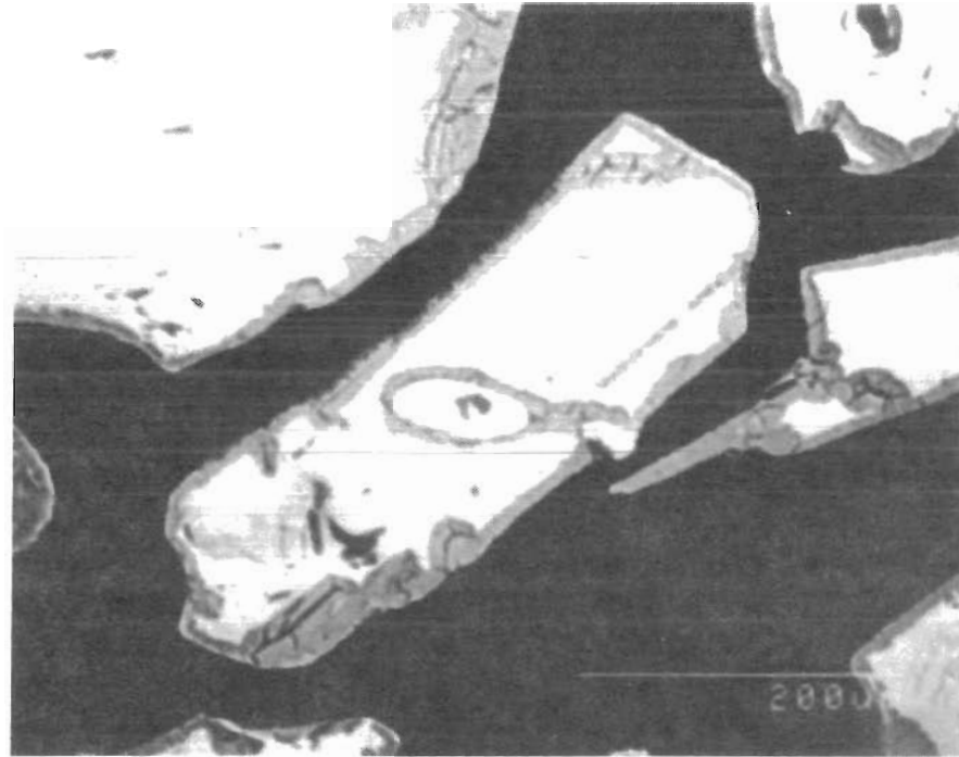
Photomicrograph of leached CdTe wafer scrap showing tellurium product layer surrounding unreacted CdTe core.
