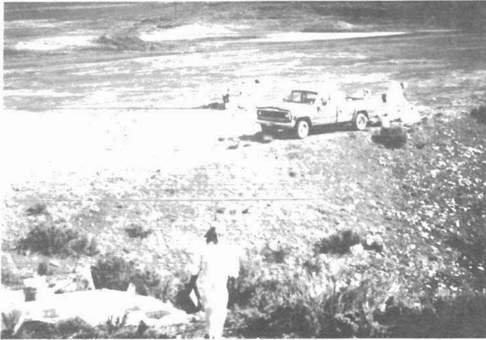
Collecting samples of Olson-Neihart tailings for second drying series in phase 1 program.
