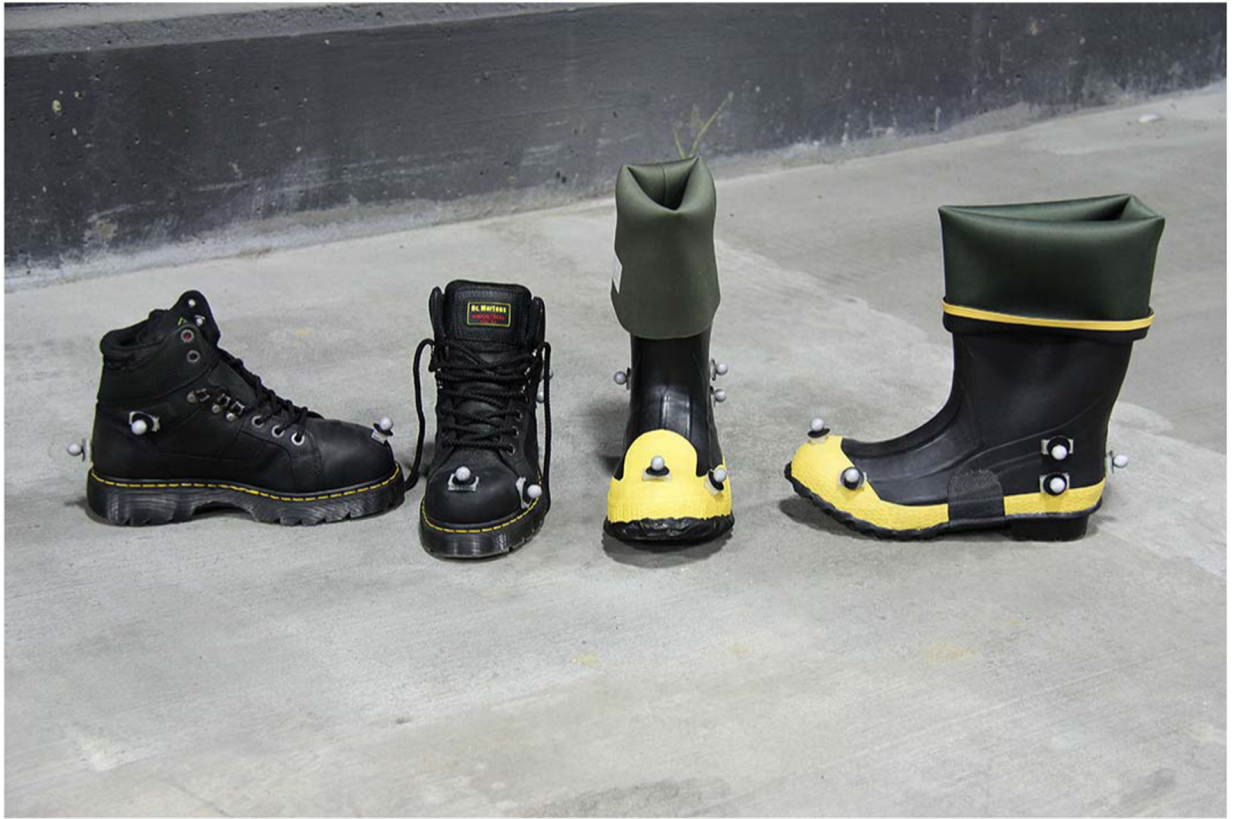
Figure 1 — Four styles of work boots worn by participants during the study, including (left to right): Hiker style with metatarsal, hiker style with steel toe, wader style with metatarsal, and wader style with steel toe.
