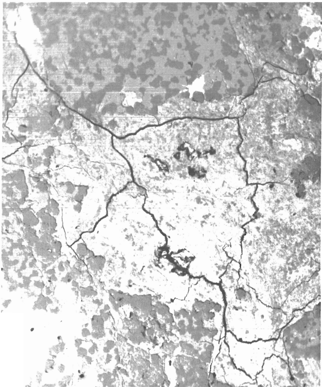
Figure 2.—Distribution of microfractures in Lakeshore copper ore.
