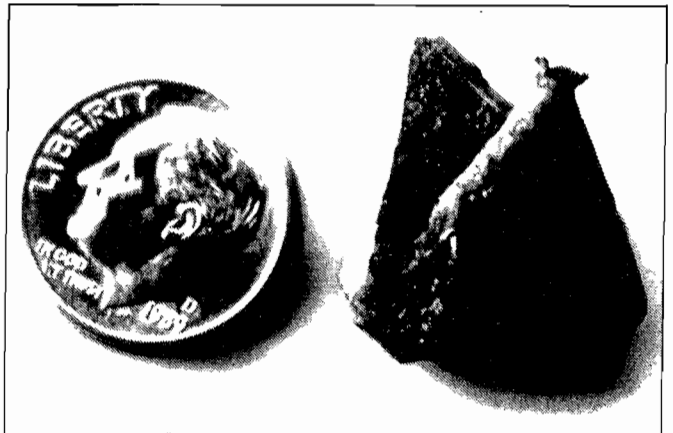
Split 19-mm taconite pebble with high-intensity arc melting at two points (95 W/cm 2 for 1.1 s).
