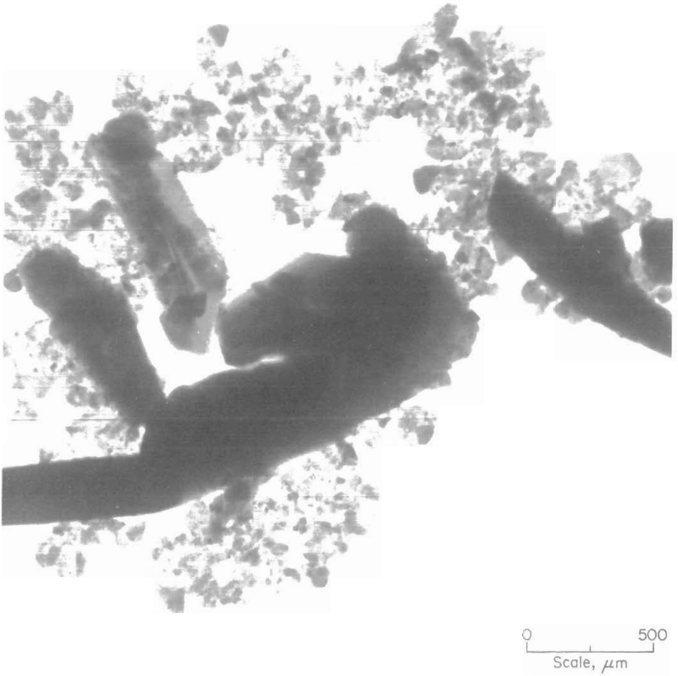
Figure 8.—TEM micrograph, orthorhombic and hexagonal phase. The octahedra are clearly visible. The dark shapes are possible hexagonal crystals viewed along the "c" direction.
