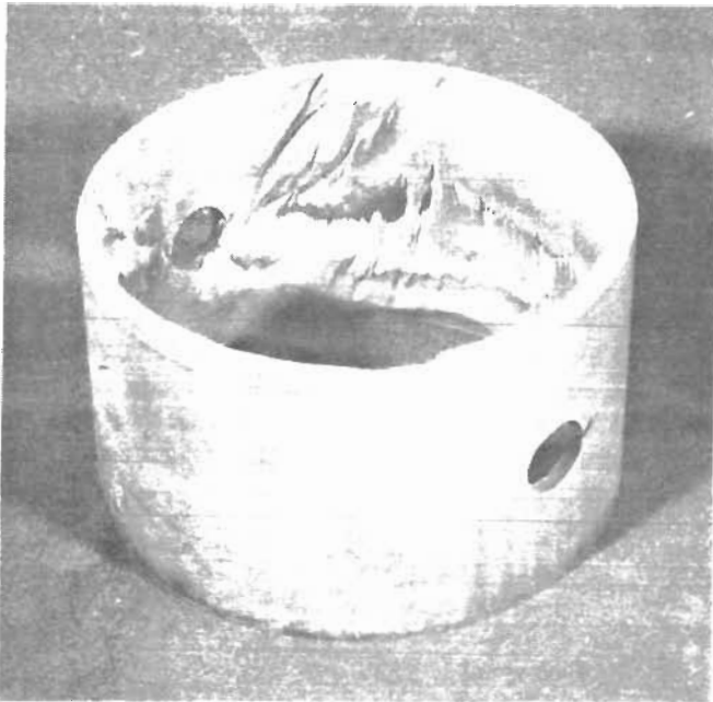
Figure 2.—Let-down valve liner damaged by entrained particle erosion.
