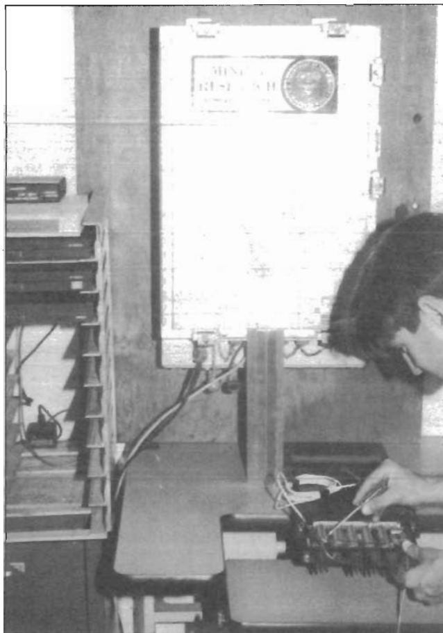
Present configuration of passive backplane system with board-level 486 processor.
