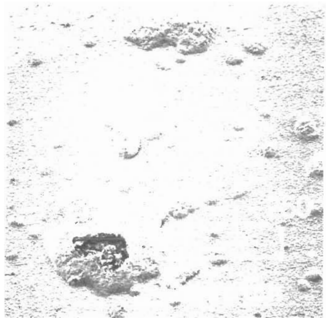
Figure 4.—Annealed coupon showing impending failure of protective Cr 2 O 3 layer.
