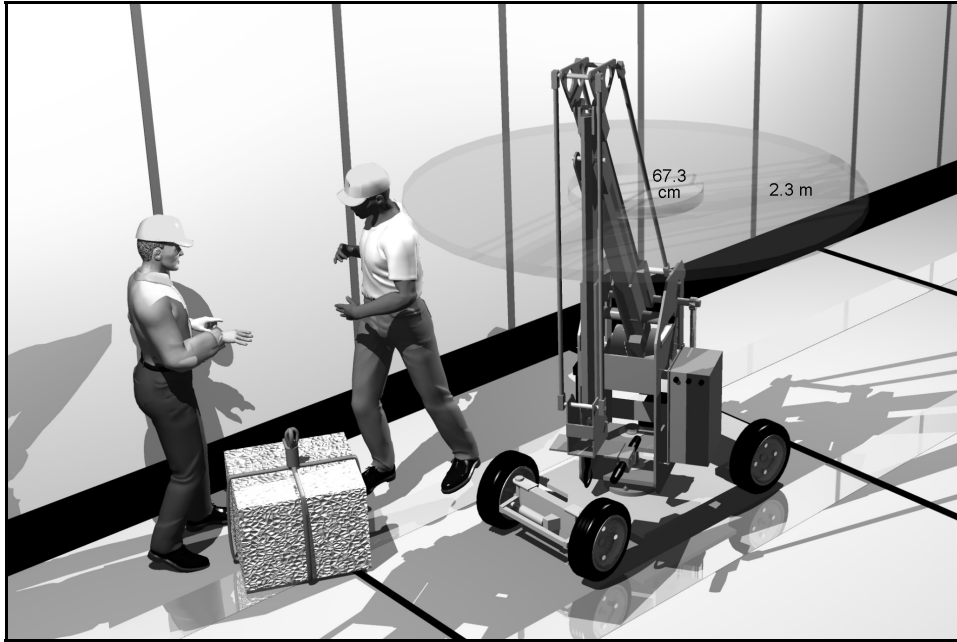
Figure 6.– Artist's concept of mobile manipulator after modifications.
