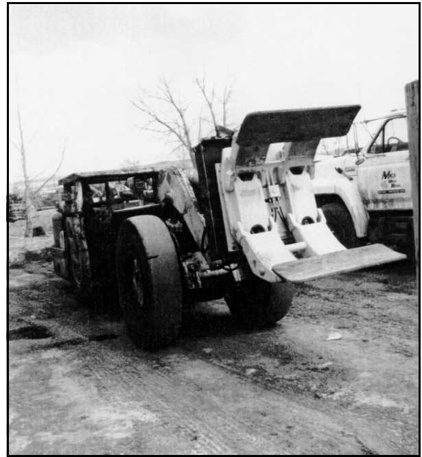
Figure 2.— Attachment used to pick up and maneuver can cribs.
