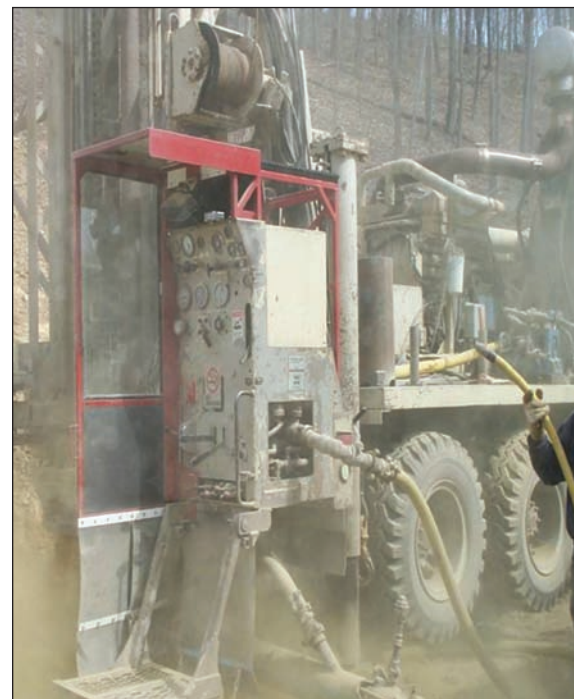
Figure 2. In field tests, the partial cab reduced the sound level at the operator control panel from 104 to 96 dB(A). Coupled with continued use of personal protective equipment, such as hearing protection devices, the partial cab can help reduce noise exposure.
