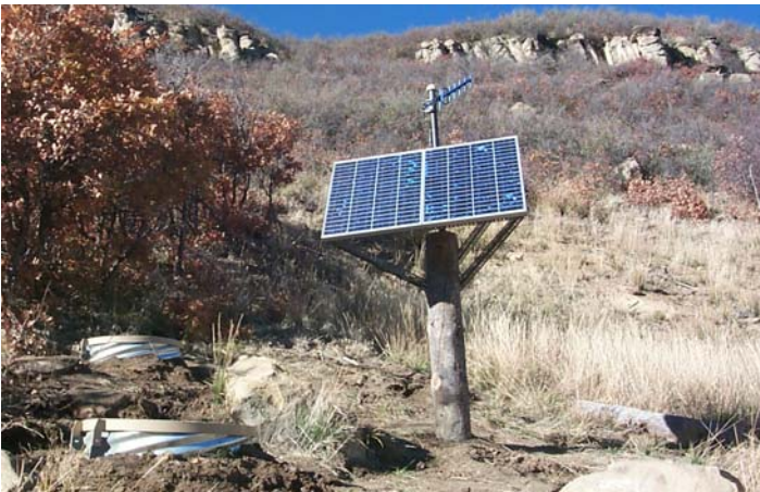
Figure 6: Remote seismic station installation
