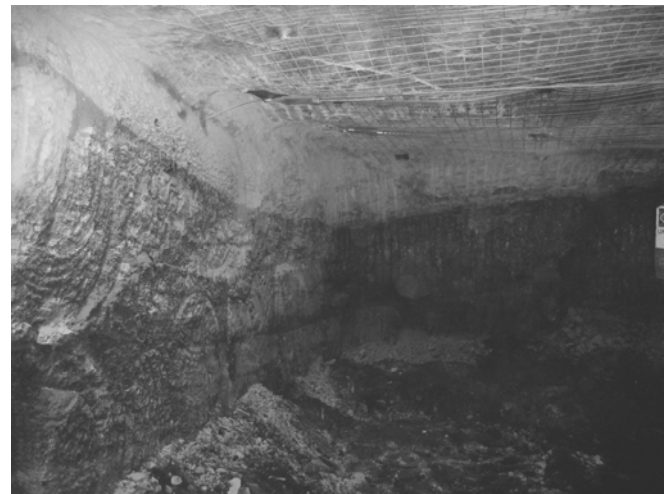
Figure 6. Photograph of a slump feature encountered in the Upper B Seam gate entry development.
