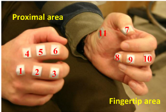
Fig. 4. Measurement locations on the fingers on the two hands and a pictorial view of the right hand holding the handle in the measurement.
