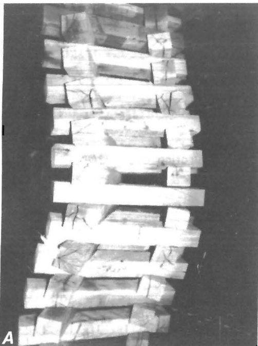
FIGURE 12.—Profile of crib structure during failure. A , Without horizontal displacement; B , with horizontal displacement.
