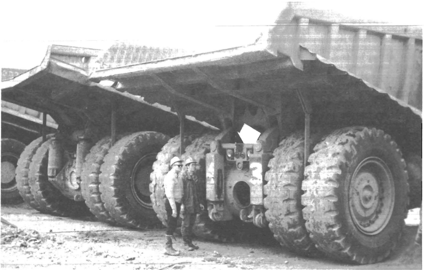
Figure 4.—Mounting location of rear receiving antenna for Telemotive system.
