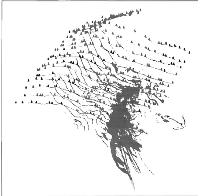
AutoCAD-software-generated surface and subsurface model showing linked cross sections and geometry of Greens Creek Mine, looking south.
